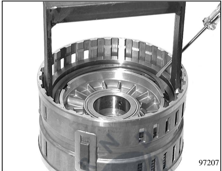
Turn cylinder D/E around, disengage the snap ring of brake E and remove the complete disc set.
