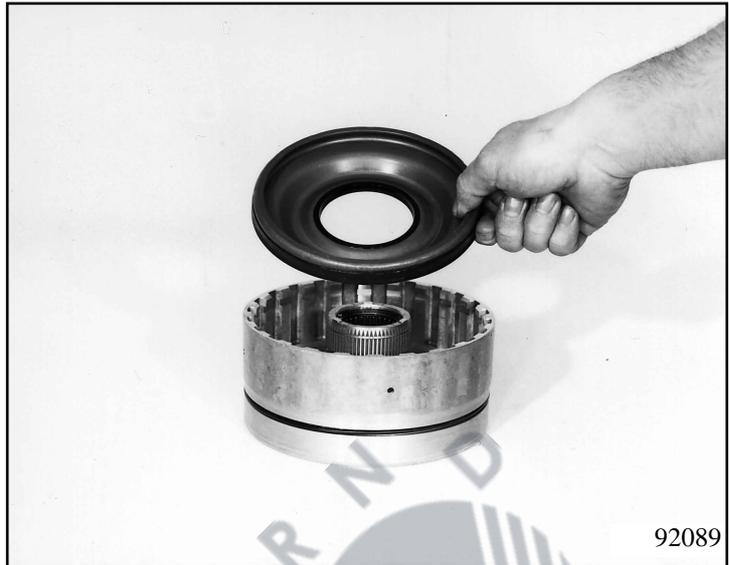
Insert cup spring 75.050, press down in the mandrel press with installation bracket 5x46 000 931 and install divided stop ring 77.060.
