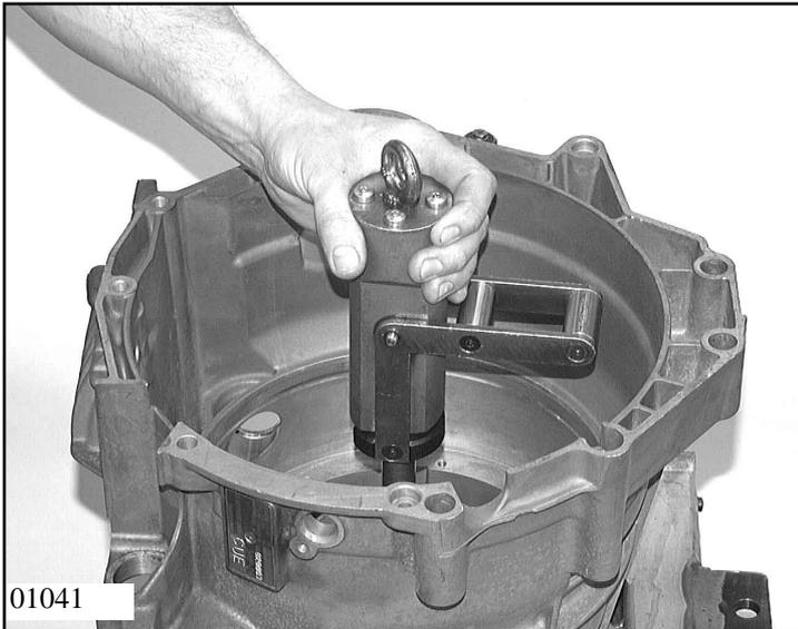
Remove tower II (input with clutches A and B).
