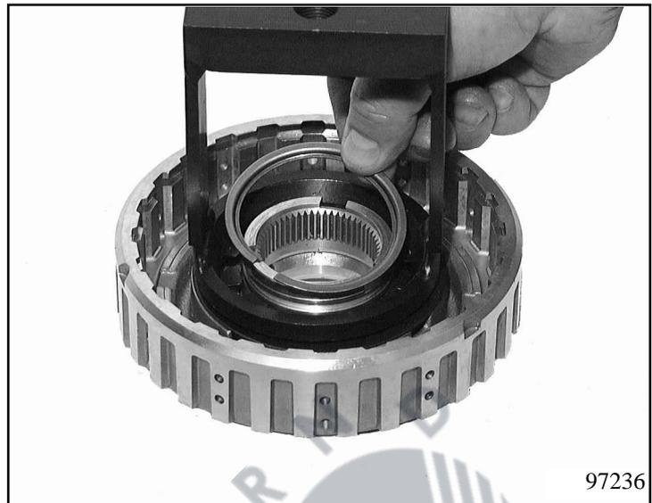
Insert complete disc set C starting with spring disc 75.010/170 followed by outer clutch disc 75.010/180 and lined clutch disc 75.010/190. Secure upper outer clutch disc 75.010/200 with snap ring 75.010/210.
