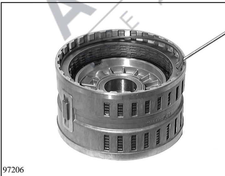
Using installation hoop 5x46 001 501, press down the cup spring C in the drift press, take out the snap ring and remove the cup spring.
