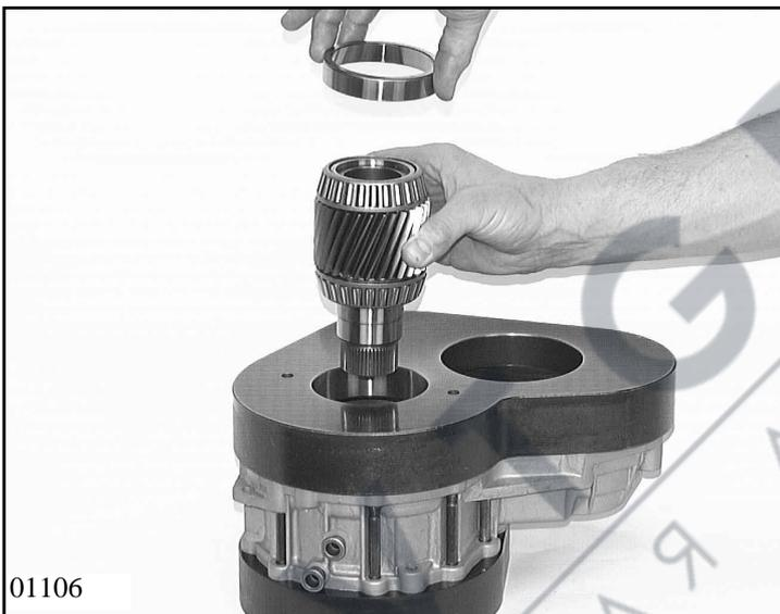
Turn the intermediate housing by 180°. Place the front axle shaft in the intermediate housing in the correct installation position.
