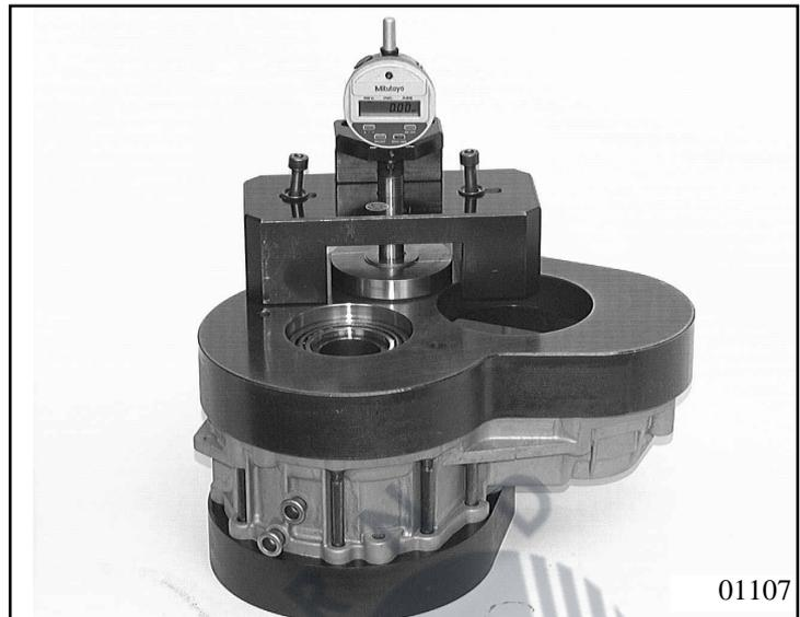
Place thrust bell on the front axle shaft outer race.
