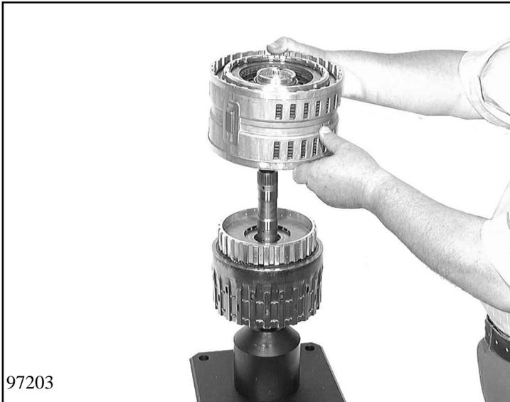
Take out clutch C with sun gear shaft.
