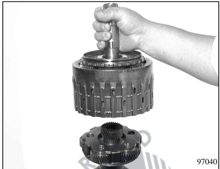
Dismantle planetary gear set III by taking the sunwheel out of planetary gear set III.
