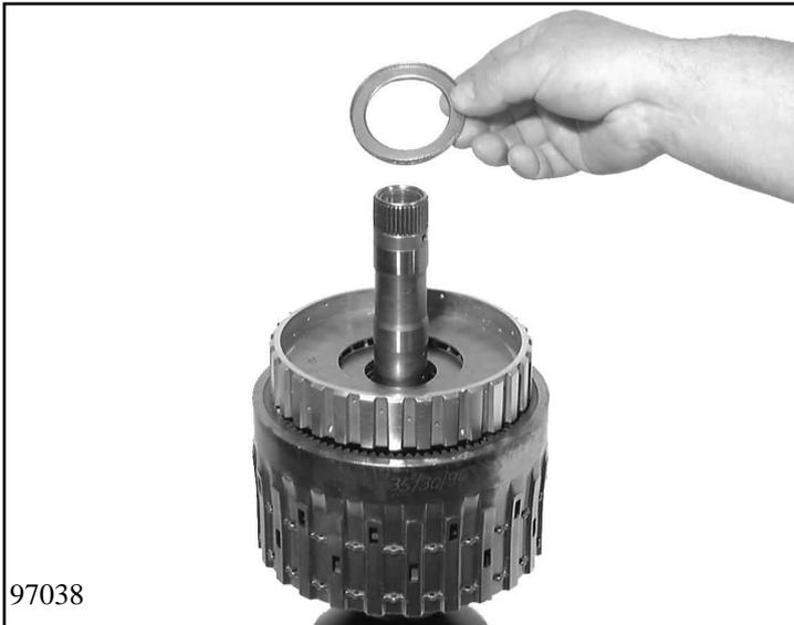
Lift off the axial needle roller bearing.
