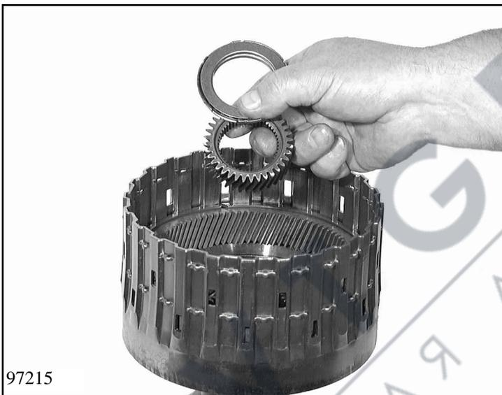
Take out the axial needle roller bearing and the sunwheel.
