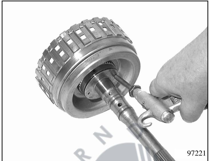
Remove the O-ring and the two rectangular-section rings from the input shaft.
