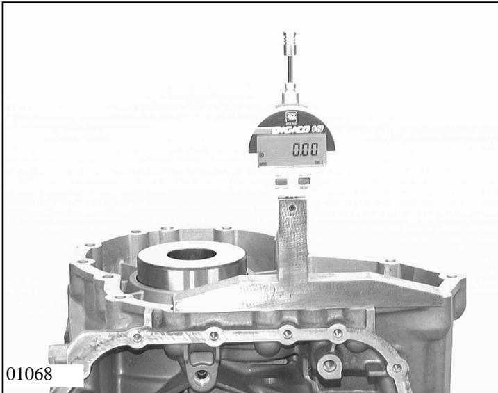
Insert measuring ring 5p01 002 889 in front axle shaft bearing hole.
