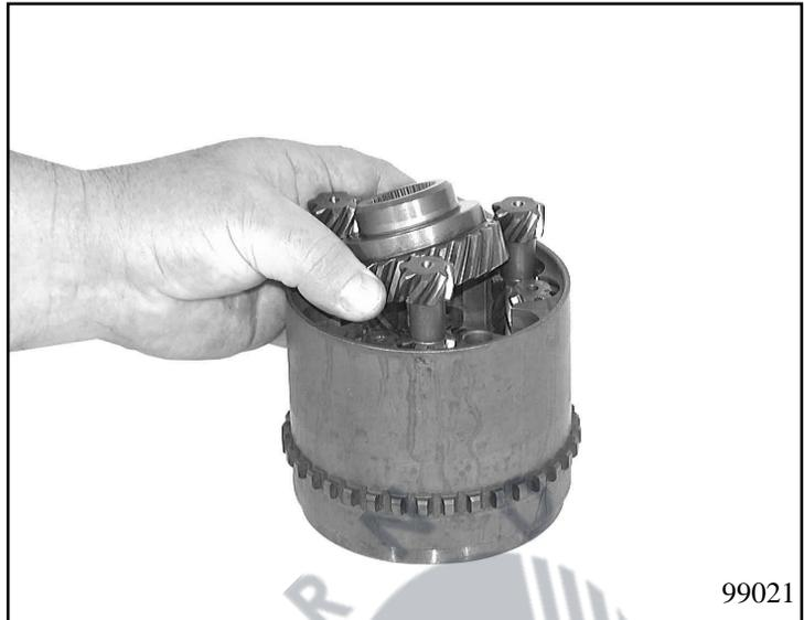
Screw in three screws at least 5 threads through the housing into the lower cover. Place the housing vertically on the workbench. Drive the cover out of the housing by striking the screw heads lightly with a plastic-faced hammer.
