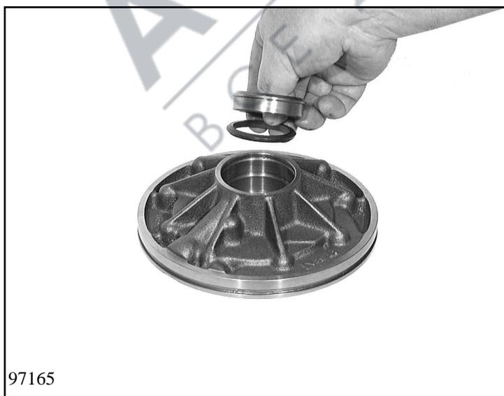
Add parts to pump 10.010; first insert sealing ring 10.010/140 into the pump housing, then press down needle roller bearing 10.010/150 in the mandrel press with installation drift 5x46 000 954.
