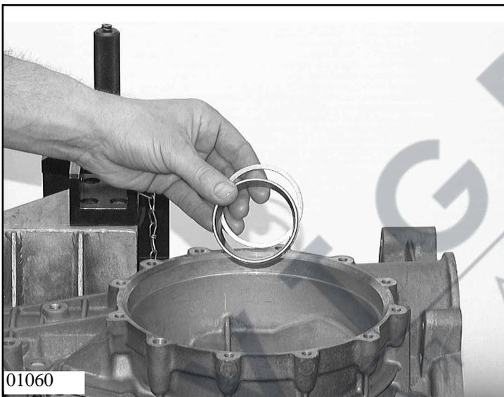
Insert the shim 35.080 previously removed into the transmission housing with the bearing race.
