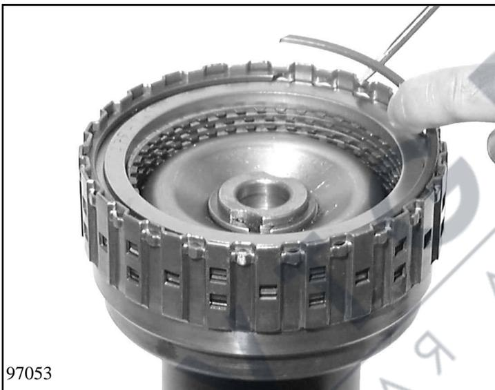
Disengage snap ring for clutch A and take out the complete clutch A disc set.
