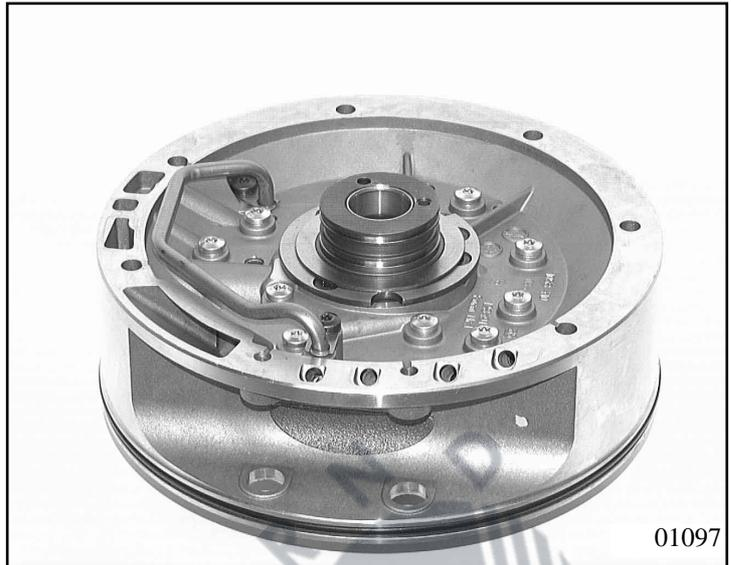
Place axial needle roller bearing 02.250 over the input shaft on clutch B.
