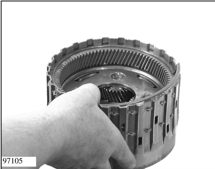
Insert ring gear III 32.240 with the outer driving splines upwards and secure with snap ring 32.250. Raise ring gear I slightly for snap ring installation.
