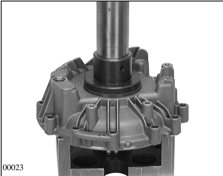
Place differential cover 35.150/110 on guide plate 5x46 001 255 and press shaft sealing ring 35.150/120 into the differential cover in the mandrel press, using drift 5x46 001 255.
