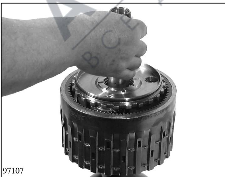
Place planetary gear carrier on the planet carrier while turning it.
