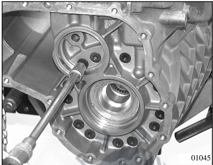
Turn the transmission through 90° and insert lifting fixture 5x46 000 831 into cylinder F by lifting the bracket handle. Releasing the bracket handle locks the fixture.
