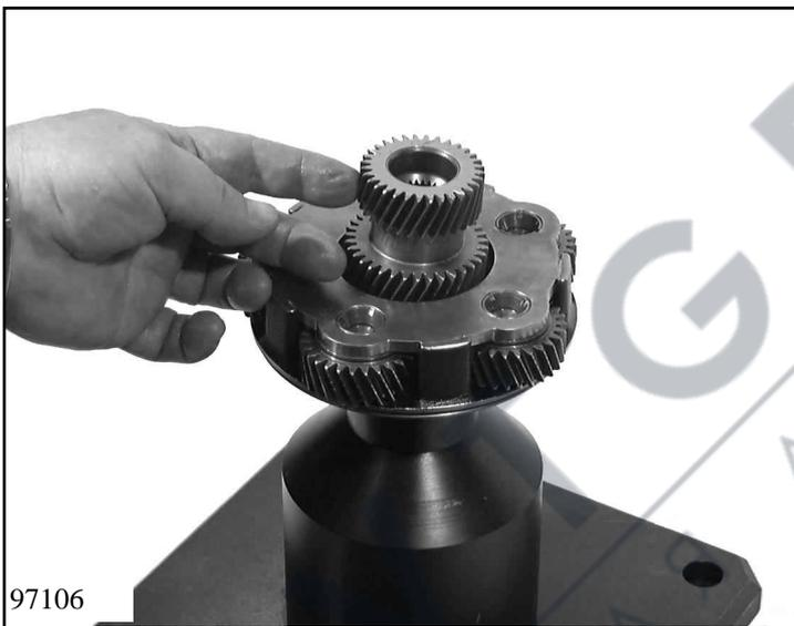
Lift planetary gear set (I and II with ring gear III) away from the fixture. Place planet carrier III 42.010 on the fixture and insert sun wheel 32.360.
