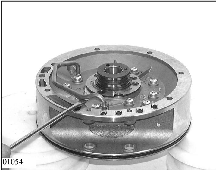
Place the entire oil supply unit on a suitable surface. Take the 2 rectangular-section rings off the stator shaft. Slacken off the 2 screws from the oil retaining plate and remove them with the plate. Using a suitable tool, lever out the oil pipe.
