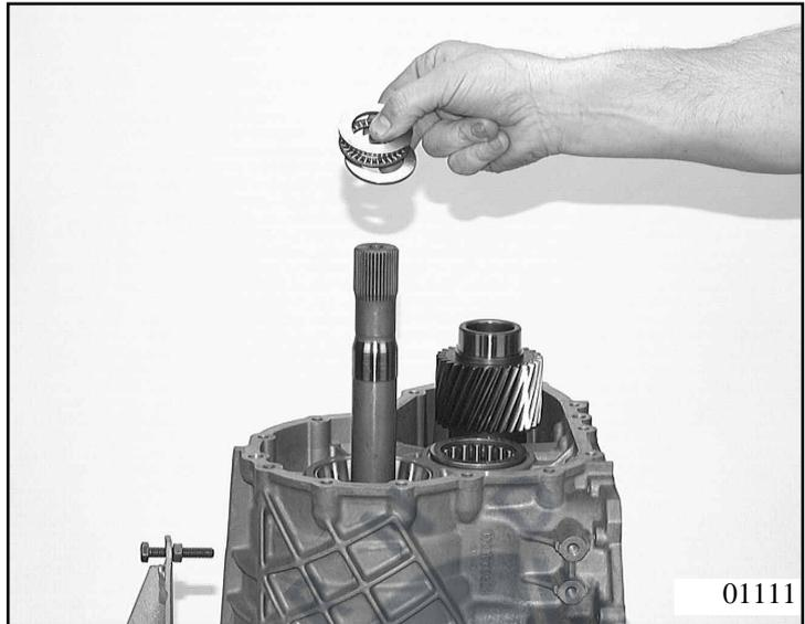
Install the front axle shaft and the intermediate gear together in the transmission housing.
