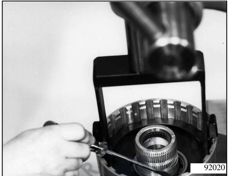
Press the piston out of cylinder F with the aid of two plastic drifts.
