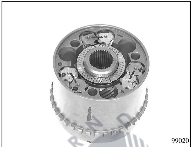
Insert three screws and tighten them initially by hand. Clamp retaining fixture 5x46 002 262 into the vice. Place the Torsen II unit in the retaining fixture with the screw heads uppermost. Tighten screws uniformly so that the covers do not tilt. Remove Torsen II unit from the retaining fixture. Check the Torsen II unit for free rotation by turning the front or rear axle shaft.
