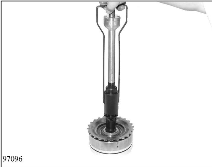
Insert lifting fixture 5x46 000 831 into brake F so that the three recesses at the collar of the lifting fixture engage with the three raised areas on the cylinder hub.
