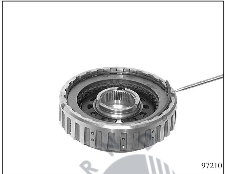
Using installation bracket 5x46 030 167, press down cup spring C in the drift press, take out the divided retaining ring and remove the cup spring.
