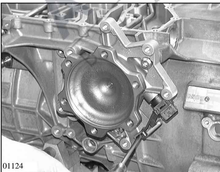
Pull two new O-rings 35.230/020 on to speedometer sensor 35.230 and press this into the speedometer housing so that the arm engages in the housing.
