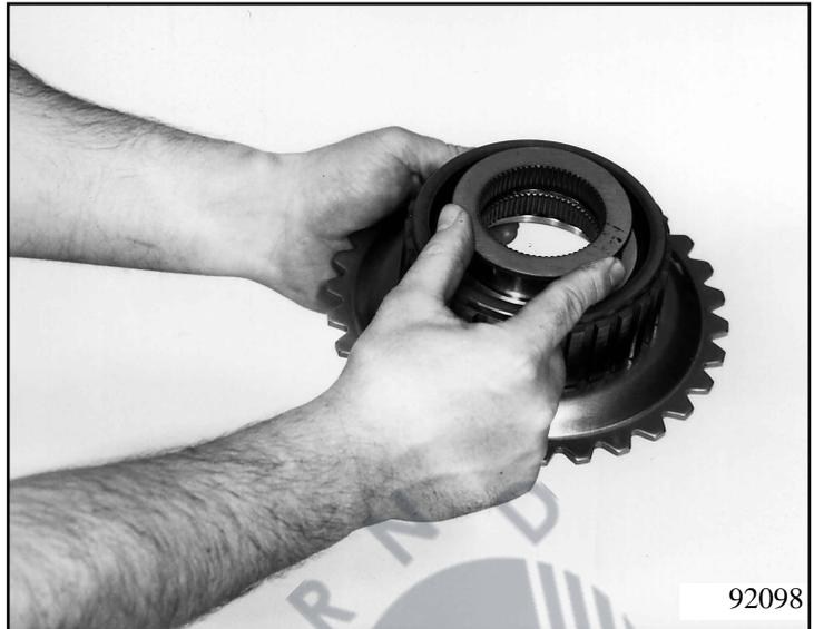
Press in stop disc 77.120/140 and secure with snap ring 77.120/150.
