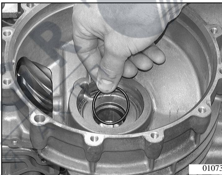
Install the correct shim washer 35.080 in the transmission housing with the outer bearing race. Insert the complete differential.
