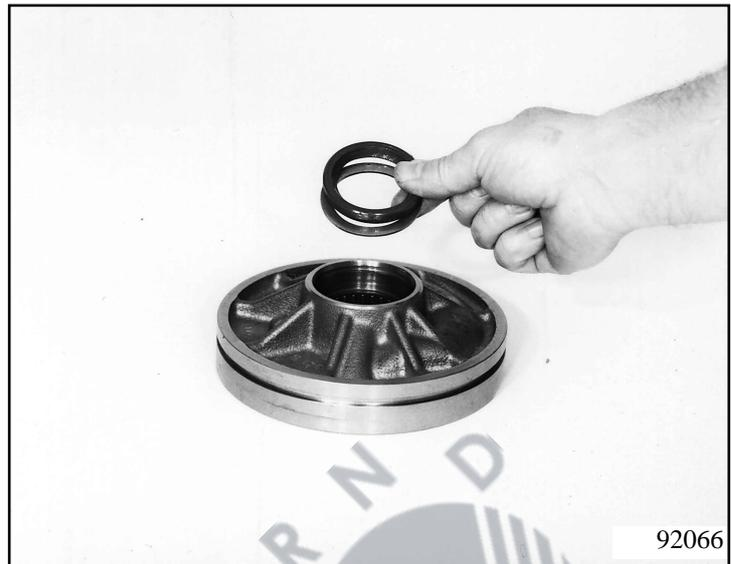
Press out the sealing ring with the needle roller bearing in the mandrel press. The diameter of the pressure pin is 42 mm.
