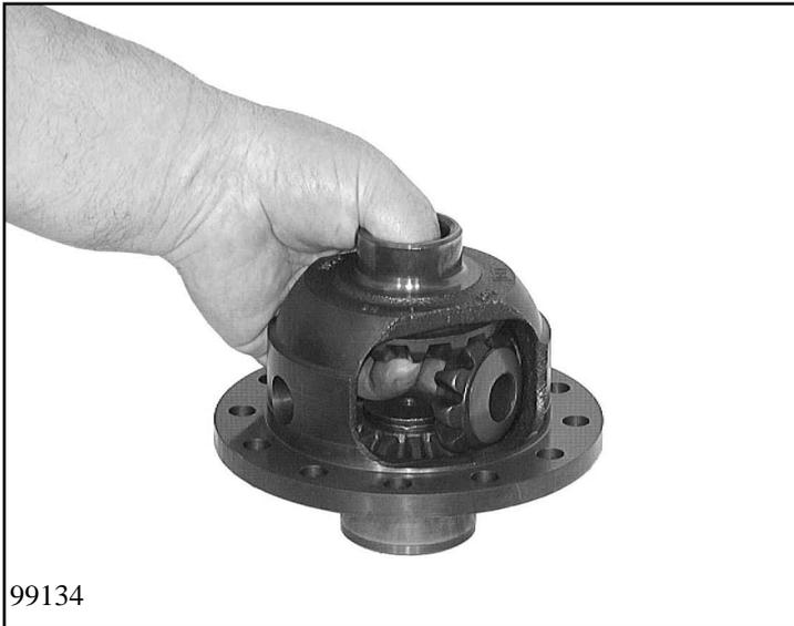
Install lower bevel gear with flange retaining and shim washers and upper bevel gear with shim washer into differential cage through inspection hole. Raise the upper bevel gear and insert the planetary gears with thrust washer through the inspection aperture. Turn the planetary gears through 90° round the differential axis and locate in position with the pin.
