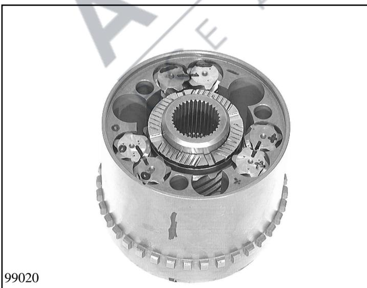
Mark planetary gear pairs, e.g. draw suitable circles, crosses or lines on the front with an electric scriber. Mark the teeth and tooth gaps of the planetary gears that are in engagement with a line.
