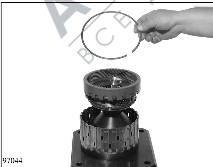
Disengage the snap ring and the divided planet carrier I from ring gear I with ring gear II.
