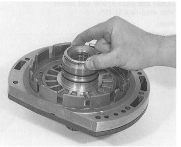
Pull O-rings 31.030 and 31.040 on to piston C 31.050, and grease lightly (with Vaseline).
