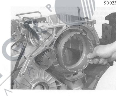
Remove the retaining screw fully. Pull the spur gear and shim washer off to one side and the side shaft to the other.
