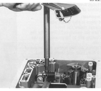
Press the new throttle cable 06.160 into the transmission housing.
