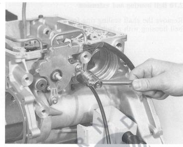
Disconnect the throttle cable from the cam and, using two suitable screwdrivers or a 10 mm socket wrench, press out the throttle cable connector.
