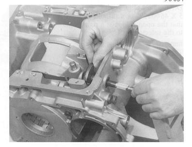
Place detent disc 06.100 on the pin; the detent spring must be pressed outwards to do this.
