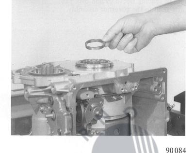
Insert washer 09.024 and place spur gear 09.020 on the side shaft. Insert screw 09.030 without tightening fully.
