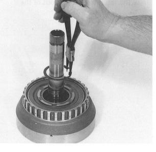
The turbine shaft can now bel pulled out towards the drive end.
