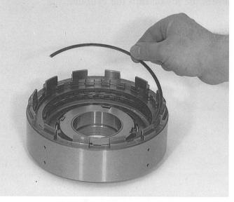
Install the complete clutch B, turning to and fro until the plates engage with each other fully.
