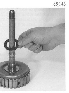
Release the snap ring and take out the complete plate cluster.
