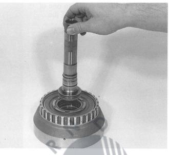
Remove the snap ring from the cylinder and take out the complete plate cluster including the spring plate. **Important: mark the plate cluster.** (The lined plates can easily be confused with brake D.) 85143
