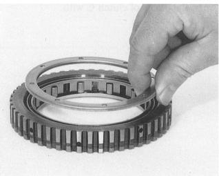
Insert the inner race of the freewheel from the front, turning clockwise at the same time.
