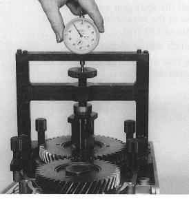
Now turn the spindle back the other way until a slight pressure point is again encountered.
