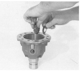
Insert differential spider 09.090/210, then install the pins in the following order: Short pin 09.090/180 (push right through) Long pin 09.090/200 Short pin 09.090/180.
