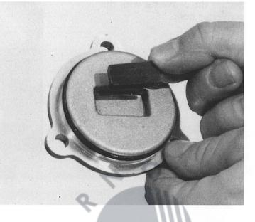
Attach the cover with 3 machine screws 01.100 and tighten the screws.
