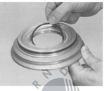
Press piston A into cylinder A 02.060/110 and insert the cup spring 02.060/140 with the curve facing upwards.
