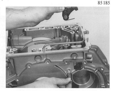
Force out the shaft sealing ring with a suitable drift.
