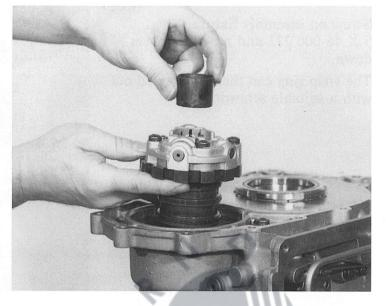
Turn the transmission through 90 degreess and remove the keeper plate from the slotted nut. Unscrew the slotted nut with wrench 5 X 46 000 155.
