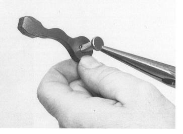
Insert the pin together with the locking cam in the segment, turn the complete assembly over and place washer 24.040 over the pin.
