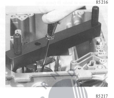
Use a feeler gauge to determine distance X between housing and cam.
