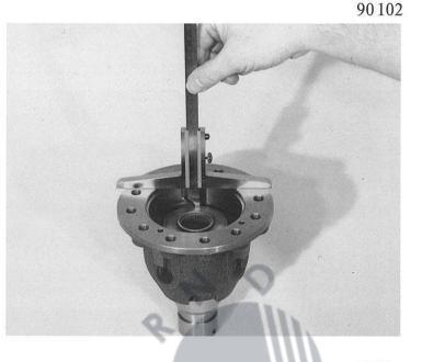
In the same way, determine distance B between the contact face and the hub of the differential cover. Example: distance B = 20.5 mm. 90103
