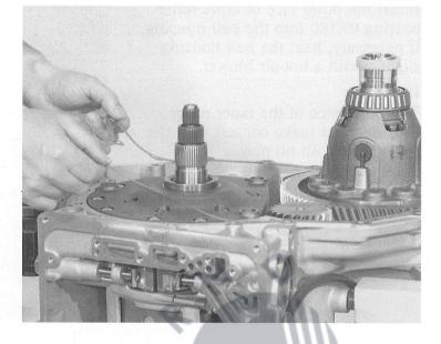
Attach the bell housing and secure it with the 18 hex bolts (Wrench size = 13 mm.) (Tightening torque = 23 Nm.) Insert screws 22.142 to secure retaining plate 22.146.
