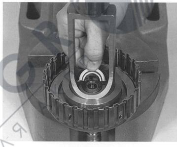
Place the two cup springs 30.080 on the piston, press them down with assembly fixture 5 X 46 000 148 in the arbor press and secure them with the divided retaining ring 30.090.
