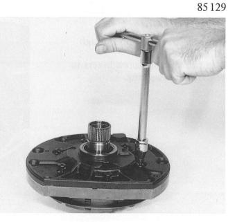
The pump can be dismantled by taking out the impeller and annulus.
