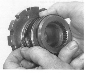
Lever off the speedometer drive worm with a screwdriver.
