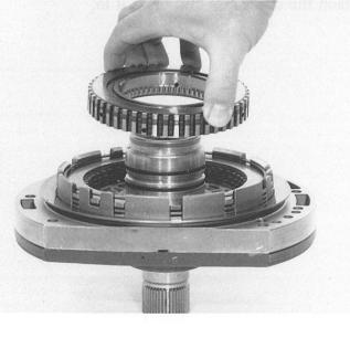
Attach the complete freewheel with the internal splines at the top to the hub of cylinder B.
