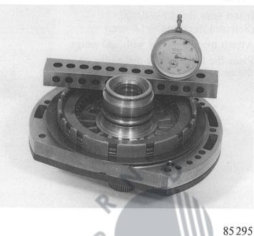
Raise the complete clutch pack and read off the play at the dial gauge. The clearance should be 1.4 - 1.6 mm.
