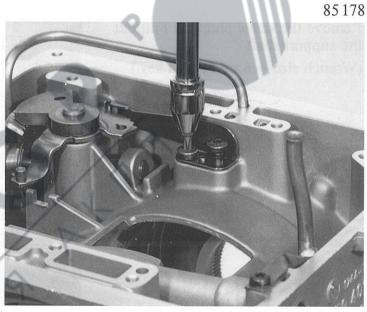
Detach the complete detent disc from the pin.
