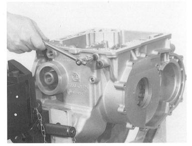
The locating pin and the pipe (external turbocharger feed) normally remain in the transmission housing.
