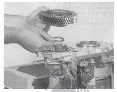
Place the gauge ring of measuring fixture 5 P 01 001 458 on the inner race of the output shaft taper roller bearing.
