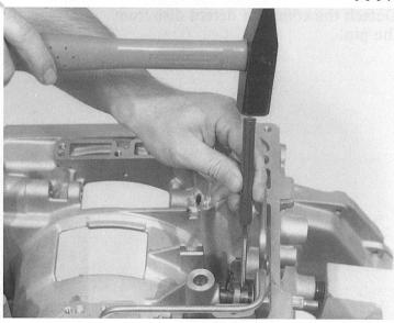
Press the pawl down slightly and take out the segment with locking cam and shim washer.
