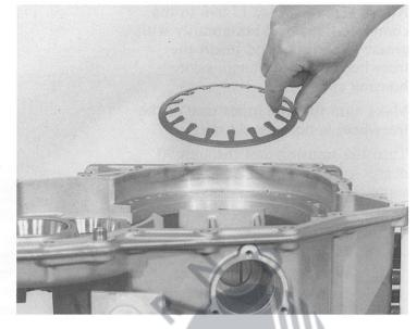
First install the two outer races of taper roller bearings 14.050 in freewheel inner race 17.160. To do this, heat the freewheel inner race to app.  $70^{\circ}$ C.
