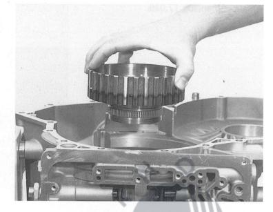
Attach keeper plate 17.170, with the retaining lug in the transmission housing. Screw on slotted nut 17.180 and tighten it with wrench  $5 \times 46 \ 000 \ 155$ .
