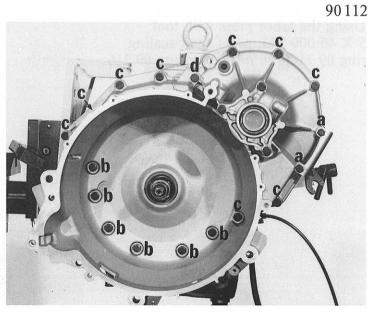
Insert the outer race of taper roller bearing 09.180 into the bell housing. If necessary, heat the bell housing slightly with a hot-air blower.
