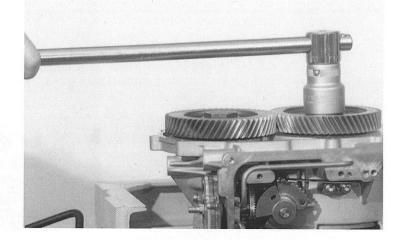
Turn the transmission through 90 degrees and release the parking lock.
