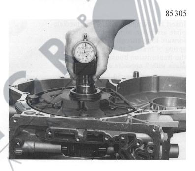
Pull the measuring fixture to determine the amount of endplay. Endplay should be 0.1 - 0.3 mm. If the measured value differs, insert a correspondingly thinner or thicker washer.
