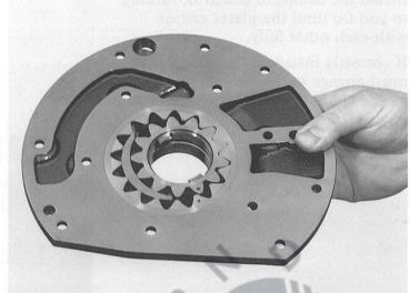
Drive two dowel pins 22.040 into intermediate plate 22.030 with a plastic-faced hammer.
