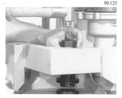
Cover 09.300 for the spur gear drive can now be installed. First attach gasket 09.290 with grease (Vaseline) and align it, then secure the cover in position with the 13 machine screws 09.310.
