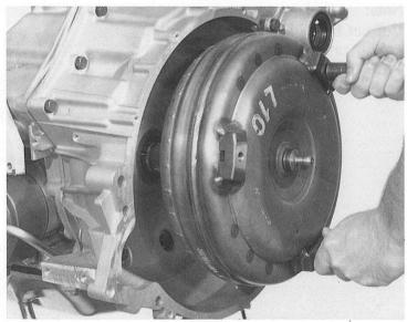
Secure the converter with the converter hoop.
