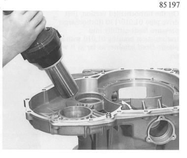
Coat the new shaft sealing ring 06.010 with Vaseline (petroleum jelly) and drive it in with assembly arbor 5 X 46 000 187.
