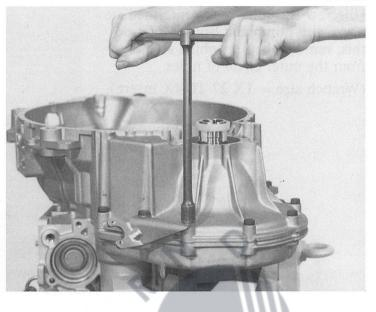
Lift off the complete bell housing. Remove the gasket.
