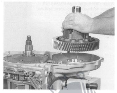
Mount speedometer drive worm 08.010 on the complete differential.
