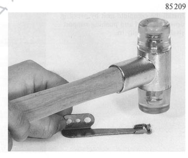
To locate pin 06.034 in the housing, press it in and attach the detent spring.
