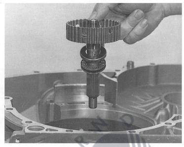
Place the two thrust washers 30.140 and the needle roller thrust bearing cage 30.150 over the intermediate shaft journal.
