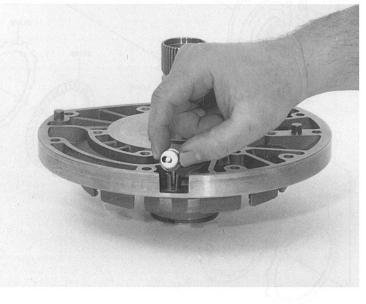
Insert coil spring 22.060 into the cutout on the pump. Attach the intermediate plate to the pump and align it.
