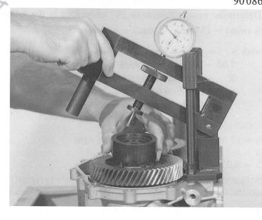
Set the dial gauge to O after having turned the spur gears at least 10 times to obtain a consistent value.
