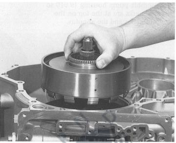
3.8 Intermediate plate with pump and brake C, 2nd gear freewheel
