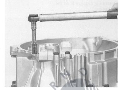
Give the retaining screw at least 10 turns to bed down the taper roller bearing.
