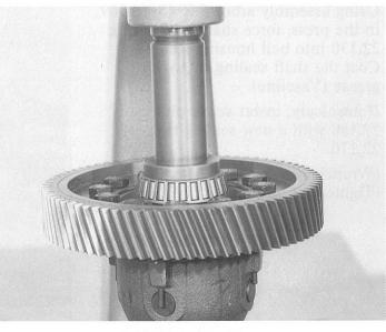
Insert the complete differential 09.090 into the transmission housing.
