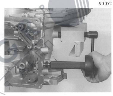
Insert torsion spring 24.060 in the pawl 24.050 as shown in this picture.
