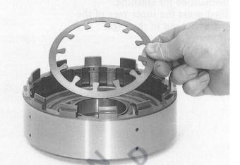
Apply a compressed air jet to the oil feed hole and press out piston B.
