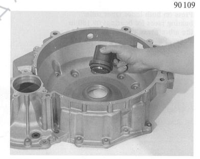
Attach seal 22.140 temporarily with grease (Vaseline) and align it.
