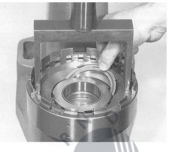
Insert the complete clutch B plate cluster, starting with outer plate 31.210, followed by lined plate 31.220 and the outer plate alternately.
