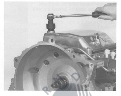
Take off the oil cooler and pipe after removing the two hollow screws. (Wrench sizes = 19 and 27 mm.) Different versions may be installed.
