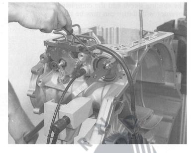
Take out the cover and complete piston C' with coil spring(s).
