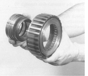
Attach retaining disc 17.090 to the complete freewheel temporarily with grease (Vaseline), and insert the freewheel into the transmission housing splines.
