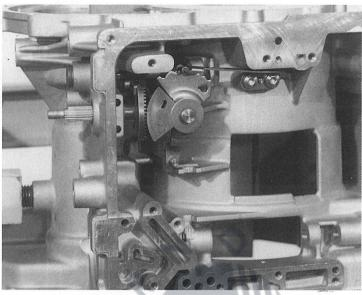
Mount switch 01.320 on the selector shaft and attach it with two screws 01.330, but do not tighten the screws fully yet.
