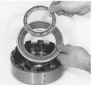
The 2nd gear freewheel can be dismantled for cleaning. First press the inner race of the freewheel out of the cage.
