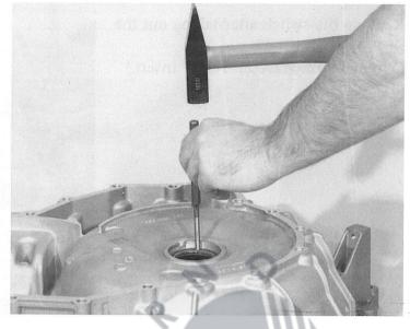
Force out the taper roller bearing outer race with a suitable drift. Take the screw plug out of the bell housing.
