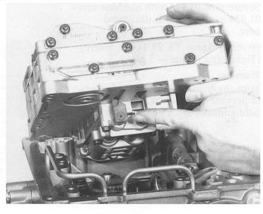
Attach control unit 200 (throttle cable pulled). Make sure that the selector valve is connected to the pin of the detent disc.
