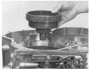
Insert thrust washer 14.020, thrust bearing 14.030 and angled disc 14.040.
