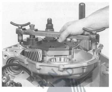
Insert the unmarked shim washer 09.090/130 and bevel gear 09.090/140 into differential cage 09.090/110.
