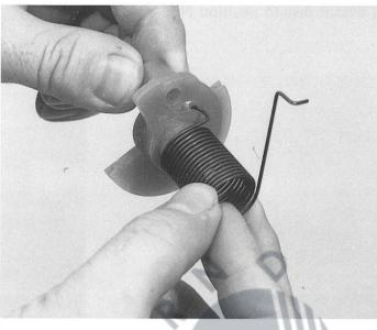
Insert throttle cam shaft 06.120 into throttle cam and torsion spring.
