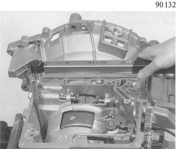
Set the detent disc to selector valve position 1 with adjusting wrench 5 P 95 000 285.
