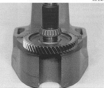
Before placing washer 14.064 on the inner race of the output shaft taper roller bearing, determine its correct thickness.
