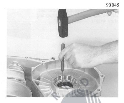
Pull out the two outer bearing races with a Kukko 21/7 or 21/8 puller screwed into basic unit 22/2. If necessary, heat the housing to app.  $70^{\circ}$ C.
