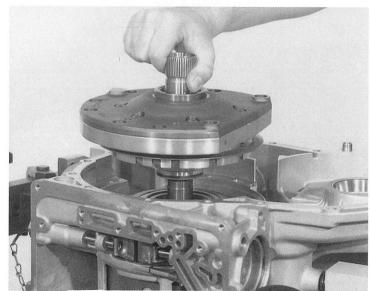
If correctly assembled, the cup spring is in contact with the transmission housing and yields when pressure is applied of the pump housing.
