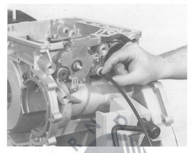
Preload the throttle cam by one turn and connect the cable nipple to the cam.
