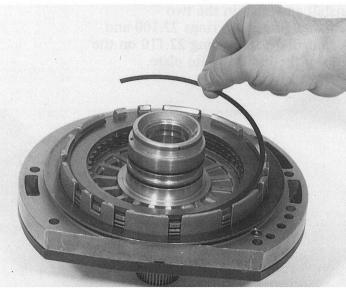
Pre-assemble 2nd gear freewheel 31.116, first pressing one of the two cover discs into the outer race of the freewheel.
