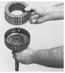
Place end plate 30.120 on the last lined plate; note that on the version with 5 pairs of plates the end plate has its turned recess facing outwards. Secure the plate cluster with snap ring 30.130.
