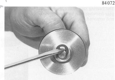
After unscrewing the locknut, the adjusting screw can be removed.
