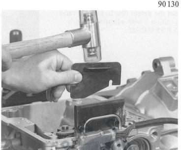
Insert oil pipe 01.120 in installing tool 5 X 46 000 280 and drive fully in with a plastic-faced hammer.
