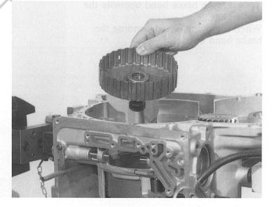
Take out the casing with axial bearing, washer and angled disc.
