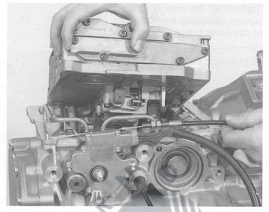
Attach the control unit with the following machine screws:
