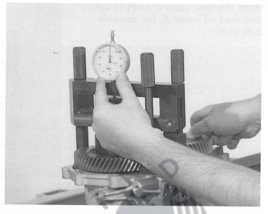
Detach preload fixture 5 P 90 000 300 from the underside of the transmission, then lower by turning the spindle adjusting screw until slight resistance is felt.
