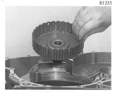
Pass angled disc 30.170, needle roller thrust bearing cage 30.180 and thrust washer 30.190 over the end of intermediate shaft 30.160, and insert the intermediate shaft.
