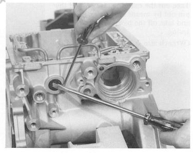
Take out the dipstick tube after removing the retaining screw. (Wrench size = TX 27 TORX insert.)
