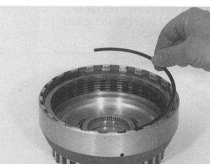
Install the two rectangular-section rings 02.040 and 02.050 on turbine shaft 02.020, and hook them into place.
