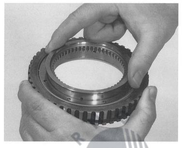
Before installing shim washer 22.090, its thickness must be determined.
