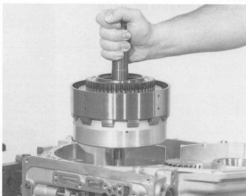
Remove the 2nd gear freewheel.
