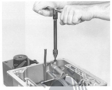
Pull out the oil pipe with suitable pliers.
