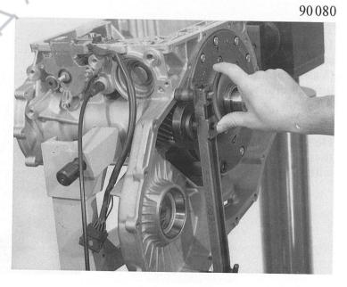
Install spacing sleeve 09.068 over the side shaft in the governor assembly.
