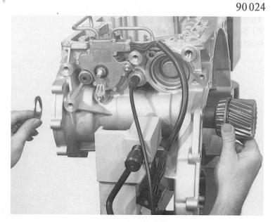
If necessary, pull the inner race of the taper roller bearing off the spur gear (output shaft) with Rollex puller 48.500, screwed into basic unit 10001, 5 X 46 000 297.
