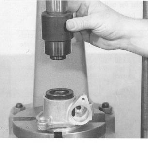
Pull on the O-ring 09.200 and coat it lightly with grease (Vaseline).
