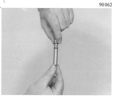
Insert the pin into the housing so that the two O-rings acts as a seal at the outside of the housing. Pre-assemble adjusting screw 31.330 with spring washer 31.340 and hex nut 31.350, and screw it halfway into the housing.
