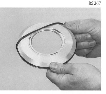
Insert the retaining disc and press it down in the arbor press, using the hoop of tool 5 X 46 000 167. Snap ring 02.060/170 can be inserted by hand, or if necessary with the aid of suitable pliers.
