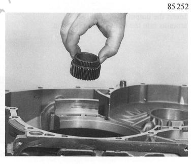
Place casing 31.290 on the sun wheel splines.
