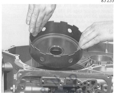
Insert thrust washer 02.230, needle roller thrust bearing 02.220 and angled disc 02.210 into the casing.
