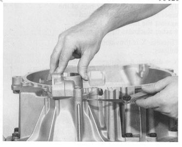
Determine washer thickness "S" according to the following formula:
