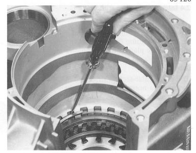
Take out the complete brake D plate cluster. Remove the cup spring. Important: mark the plate cluster to avoid confusion.
