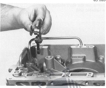
The complete unit can be dismantled by disconnecting the spring clip from the segment and pulling it out of the pin.
