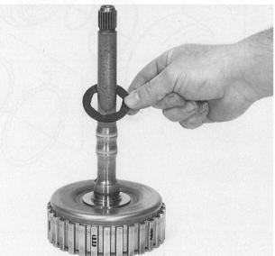
Insert the engine shaft, turning it at the same time. Make sure that all the plates are correctly engaged.
