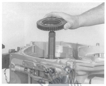
Insert the shim washer of the calculated thickness, and angled disc 22.080.
