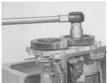
Release the parking lock and bolt on measuring fixture 5 P 01 001 458 firmly in a position that allows the pin to be pushed into the spindle loop and the centre screw at the same time.
