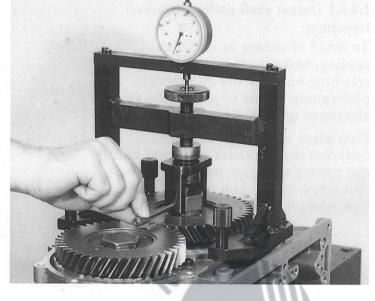
Turn the spindle of the fixture in one direction until a slight pressure point is felt.
