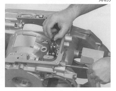
Insert screw plug 24.120 with a new sealing ring 24.110. (Wrench size = 6 mm Allen key.)
