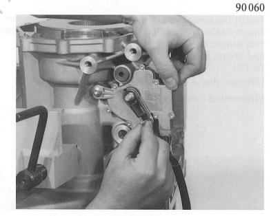
Connect torsion spring 06.130 to throttle cam 06.110 as illustrated.
