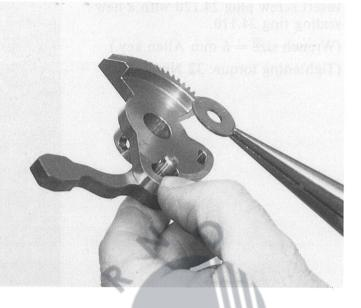
Next, insert spring clip 24.010 through the pin and connect it to the segment.
