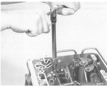
The throttle cam shaft with torsion spring and the throttle cam can now be removed.
