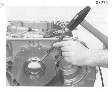
Insert the complete brake D plate cluster. Start with spring plate 17.046, followed alternately by outer plates 17.050 and lined plates 17.060. Install end plate 17.070 and secure with snap ring 17.080.
