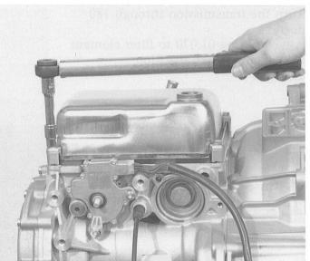
Screw breather 01.300 into the oil pan, using a new sealing ring.
