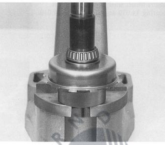
Insert the output shaft into annulus 32.040 and secure with snap ring 32.050.
