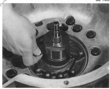
Also attach measurement gauge 5 P 01001415 onto teeth of input shaft and secure gauge with locking nut.
