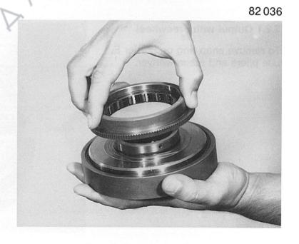
After removal of the snap ring disconnect freewheel inner ring from hollow gear.
