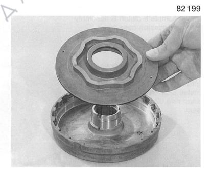
Insert plate spring 02.090 on top at piston A.
