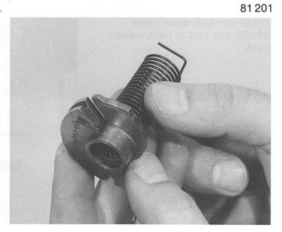
Install cam together with leg spring and insert selector shaft to stop point. Align hole in selector shaft with hole in stop washer.
