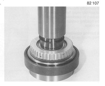
Install first steel thrust washer 30.142, second copper thrust washer 30.146 as shown in the picture.
