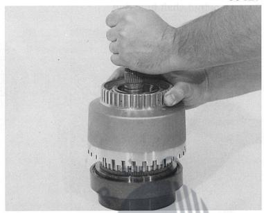
Remove axle disc and cage as well as 2 thrust washers.
