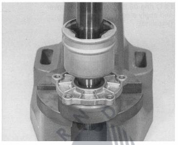
Insert tapered roller bearing outer ring 09.252 into transmission housing. If necessyra, use hot-air fan to heat up the housing a little.
