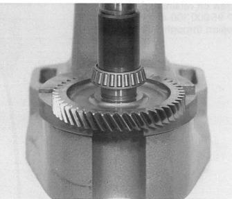
Before installing washer 14.064 onto the tapered roller bearing inner ring of the output shaft, the thickness of the washer has to be determined.
