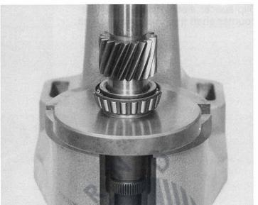
Turn transmission through 90° and insert counter shaft into the engaging gears of the governor flange while rotating the shaft and holding the flange in position to prevent it from falling out.
