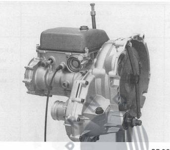
Use the 2 mounting grips 5 X 56 000 090 to take out the torque converter.
