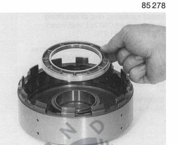
Fit new O rings 31.190 and 31.200 onto the piston B 31.180 and apply a light coating of grease (Vaseline).
