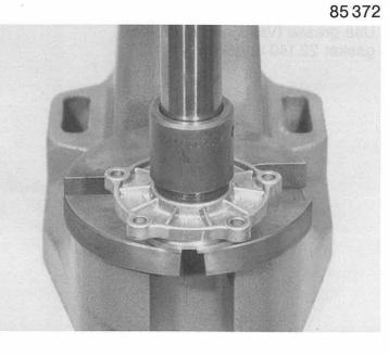
Press the left input shaft 09.250 into bearing cover under the mandrel press.
