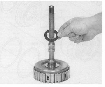
Install engine shaft while turning it. If installed correctly, the shoulder of cylinder E is flush with the edge of the disc carrier on the sun gear shaft.
