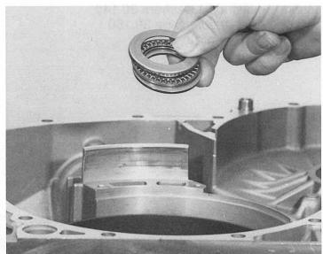
Insert axial washer 02.230, axial needle bearing 02.220 and angle washer 02.210 into the pot.
