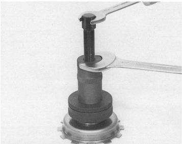
The freewheel inner ring can be pressed out of the complete unit.
