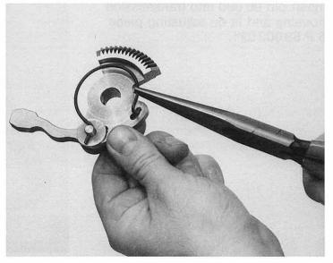
Insert complete unit by pressing down the pawl and inserting the supporting shaft 24.100 as far as it will go.
