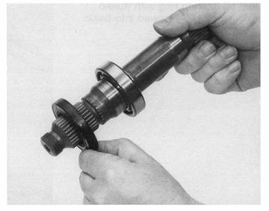
Remove locking ring from the input shaft and use special tool 5 X 46 000 314 to force off the ball bearing under the mandrel press.
