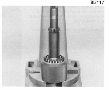
Turn transmission through 90° and withdraw bearing outer ring with the Kukko internal extractor, size 21/8, screwed into counter support size 22/2.
