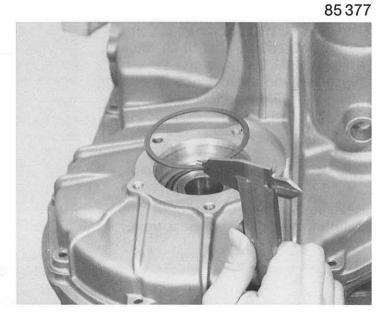
Fit O ring 09.220 onto bearing cover and apply a light coat of grease (Vaseline).
