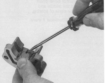
Check the rectangular and, in particular, the two Pagu rings for signs of damage. Remove if necessary.
