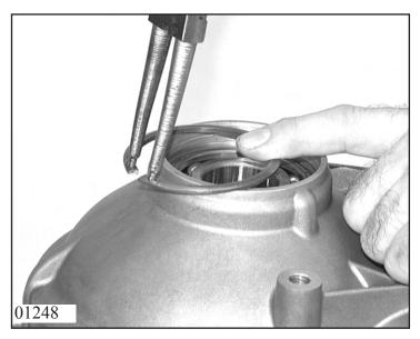
Remove the snap ring with pliers. Press the ball bearing out of the transmission casing with a suitable mandrel.
