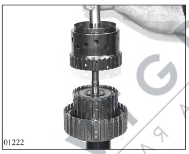
Take out disk carrier A and lever axial needle roller bearing out of intermediate shaft with a long scriber.
