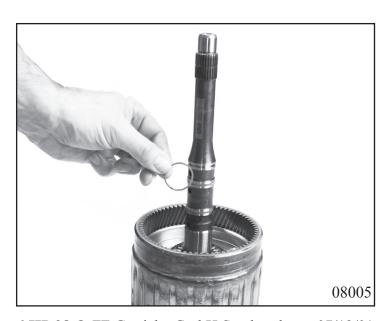
**Note!** Unclip needle roller bearing if defective.
