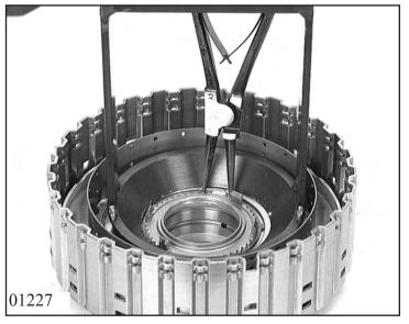
Press down cup spring in the mandrel press with assembly bracket 5x46 001 500 and remove snap ring with suitable pliers. Take out baffle plate and cup spring.
