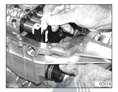
Unscrew screws with **large head** (M6) and lift off complete Mechatronics.
