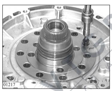
Loosen 11 machine screws (countersunk head - outer ring of stator shaft); do not take out two machine screws on opposite sides fully. Drive out the pump by striking these screws carefully with a plastic-faced hammer.
