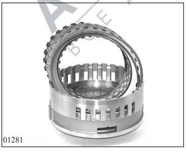
Insert complete clutch pack C into cylinder CD, starting with spring disk 75.100. Then insert an outer disk 75.140 and a lined disk 75.120 alternately. Secure the top outer disk 75.160 with snap ring 73.180.
