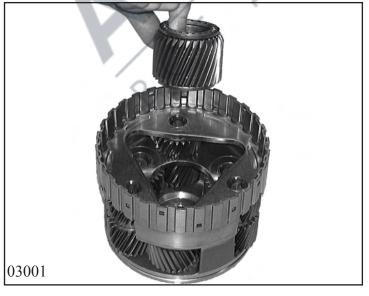
Take off sun wheel 2 from planet carrier. Clip off both axial needle bearing from sun wheel.
