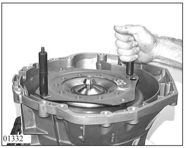
Turn transmission by 90° and move converter back and forward until the pump drive pins engage.
