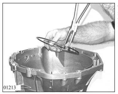
Turn transmission by 90° and lever snap ring out of casing with a screwdriver or take it out with snap ring pliers. Lift off clutch C.
