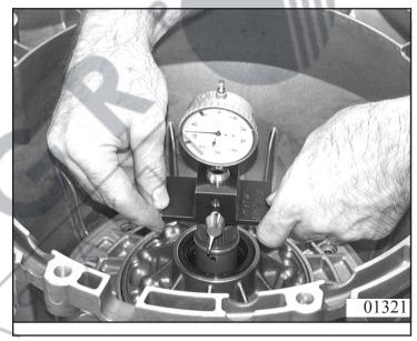
Determine axial clearance by pressing and pulling the handle (repeat measuring process several times).
