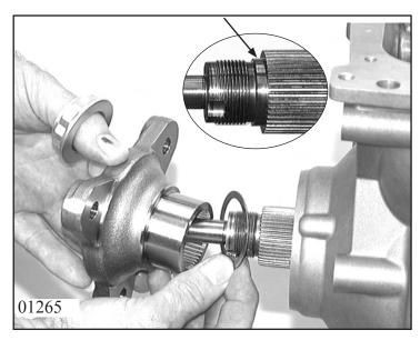
Place reversing disk 14.130 over drive shaft, push flange onto output shaft
