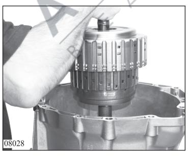
Align disks of clutch B, insert turret by hand and turning it in both directions until the disks engage fully in disk carrier B.
