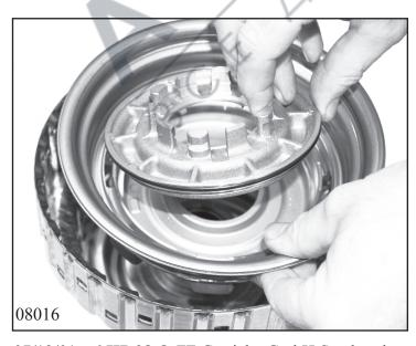
Install new O-ring seals 72.050 and 72.060 on piston B 72.020.
