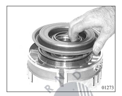
Pull one O-ring seal 73.070 onto baffle plate D 73.060.
