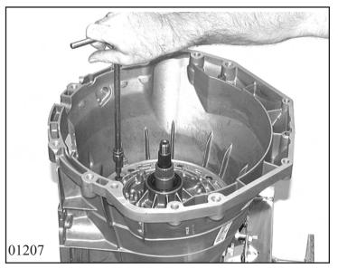
Turn transmission by 90°. Completely remove oil supply unit. To do this, loosen 14 Torx screws and remove with Usit rings.
