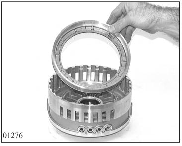
Pull two lip sealing rings 75.040 and 75.050 onto the piston C 75.030. Oil the lip sealing rings lightly and set the piston straight and press it carefully into the cylinder.
