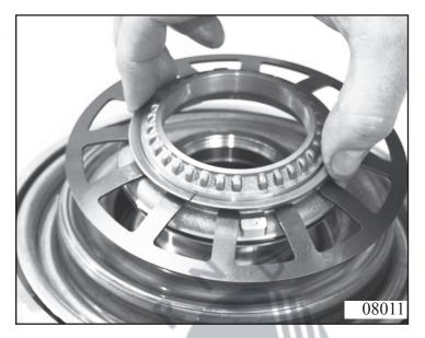
Carefully press out piston D with a compressed air supply at the oil guide bore.
