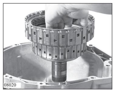
Insert angular disk 75.200 in cylinder CD and also complete clutch B into transmission housing.
