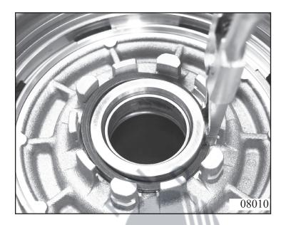
Cover one of the two oil guide bores and press out the piston, using pressurized air.
