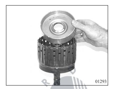
Pull new O-ring seal 71.090 onto baffle plate 71.080. Insert cup spring 71.060 into cylinder E with the projections facing downwards and press in the baffle plate.
