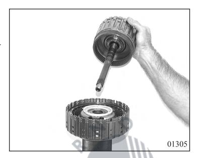
Align disks of clutches A and E. Clip axial needle Bearing 71.260 into input shaft.
