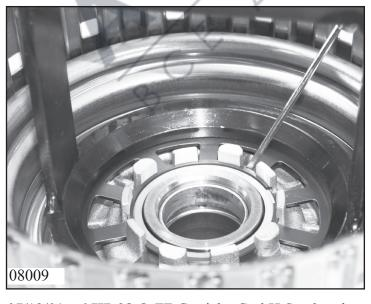
Press down cup spring B in the mandrel press with assembly bracket 5x46 001 502 and take out the snap ring. Remove washer and cup spring.
