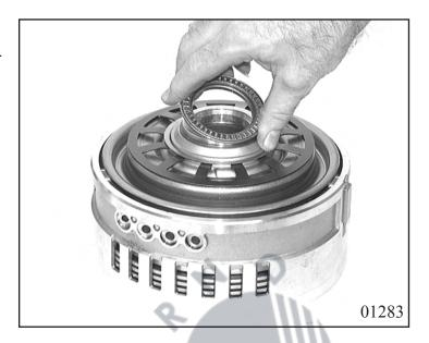
Insert complete clutch pack D into housing, starting with final disk 73.260, then insert lined disk 73.250 and external disk 73.240 alternately.
