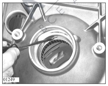
Press needle roller bearing 14.020 into transmission casing using mandrel 5x46 004 373.
