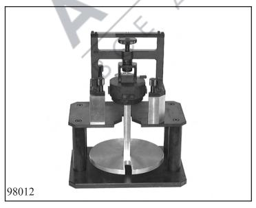
Fasten it with 4 knurled screws to the measuring fixture using the intermediate pieces.
