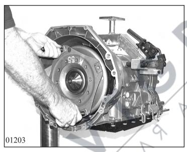
Remove converter bracket and take out converter
