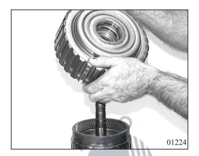
Rebound the snap ring of clutch A and pull out the complete disk set.
