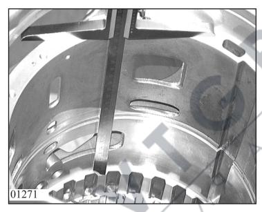
Place measuring base on cylinder support area CD in the housing and read off dimension  $\Leftrightarrow W_{DB}$ .
