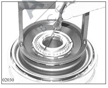
Turn the cylinder around and press down cup spring D in the mandrel press with assembly bracket 5x46 001 500; take out split retaining ring.
