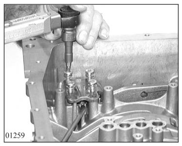
Press down ratchet and fasten guide plate 24.110 with 4 Torx screws 24.120.
