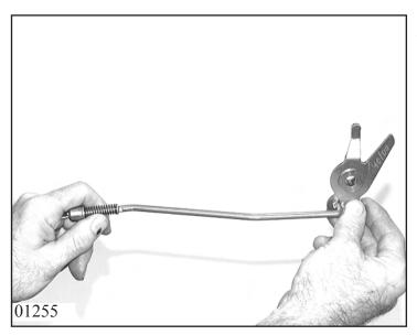
Attach connecting rod 24.080 to parking or detent disk 06.050 and turn to secure.
