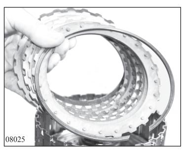
Insert the complete clutch pack E. Start with the spring disk 71.140, then insert the outer disk 71.150 and the lined disk 71.160 alternately.
