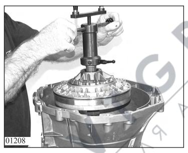
Press out the oil supply unit with jack 5x46 000 563 and lift off.
