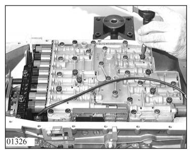
Attach parking or detent disk at groove in piston rod.
