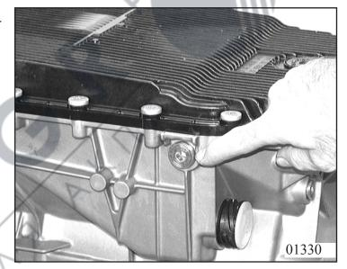
Screw in both converter handles 5x56 000 090 and carefully insert converter 22.010.
