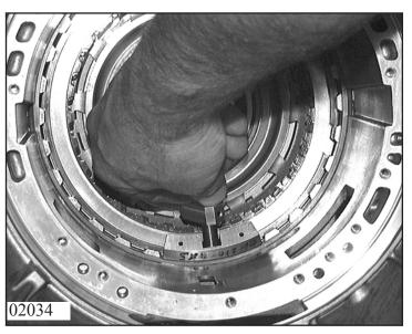
Secure with snap ring 75.260. Use driving-in tool 5x46 001 930 to drive the snap ring into the housing groove all round.
