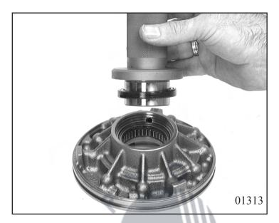
Pull on new O-ring seal 10.020. Lubricate the pump wheel and internal ring gear lightly before assembly. Then assemble the pump in such a way that one marking is visible both on the pump wheel and the internal ring gear.
