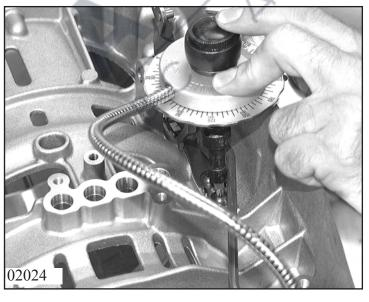
Tighten farther by the specified angle with special tool 5w04 000 583. Remove centering device. Shift the selector shaft through all positions and remove it again.
