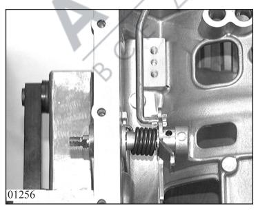
Insert parking or detent disk with connecting rod into transmission casing and push selector shaft 06.030 in through pipe 06.070 and detent disk.
