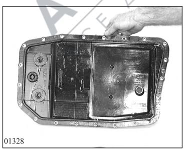
Pull new O-ring seal 03.010/020 onto stub pipe of oil filter 03.010. Press new seal 03.014/010 into oil pan.
