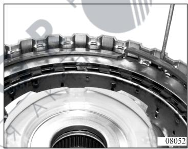
Prise out snap ring with a small screwdriver from the planet carrier at several points alongside the planet gear. At the same time raise slightly the planetary gear set.
