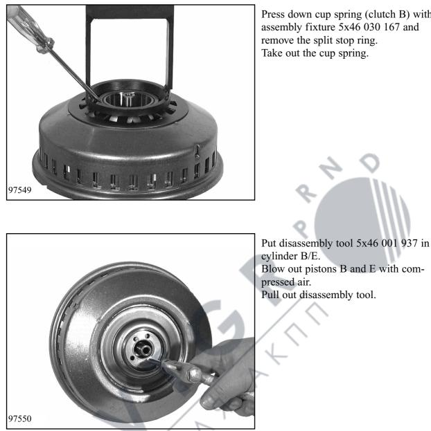
Press down cup spring (clutch B) with assembly fixture 5x46 030 167 and remove the split stop ring. Take out the cup spring.
