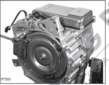
Remove converter retaining bracket with fastening screws.
