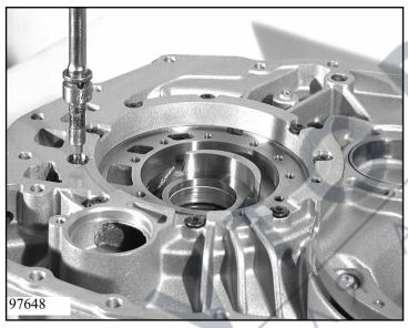
Turn the converter bell by 180° and fasten pump housing crosswise with nine screws 10.020.
