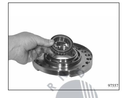
Use the Kukko internal extractor to take the bearing outer rings out of the bearing plate.
