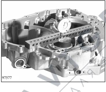
Insert plug gauge 5p89 004 177 into the side shaft bearing seat on the converter bell housing and use the measuring bar to measure down to the plug gauge from the converter bell support surface.
