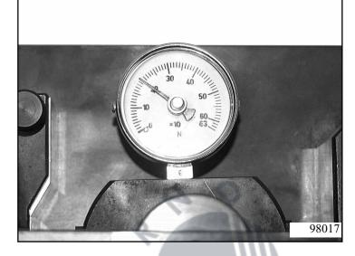
Then place measuring bar  $5p01\ 060\ 330$ on the measuring plate, put the the dial gauge's measuring base in the measuring plate's groove on the top disc of the set, and set the dial gauge to **0**. Now use the measuring bar to measure down to the base plate.
