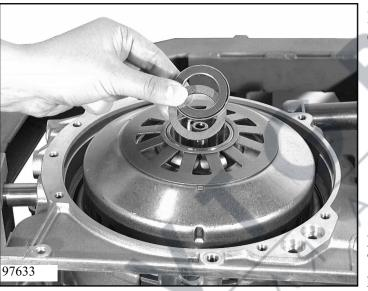
Place shim 01.100 and bearing 01.090 on cylinder B/E.
