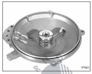
Insert two sealing sleeves 01.080 into the transmission housing; lay shim 01.100 and axial nedle roller bearing 01.090 on the hub of clutch B/E.
