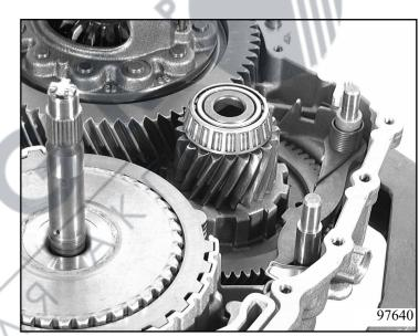
Put position switch 01.200 on selector shaft in the "N" position and screw it tight with two screws 01.210.
