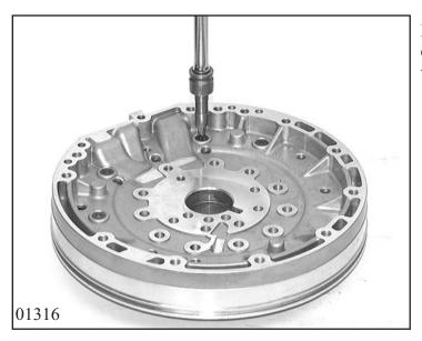
Put intermediate plate 10.040/110 on centring plate 10.040/130 and loosely fix with 4 screws 10.040/180.
