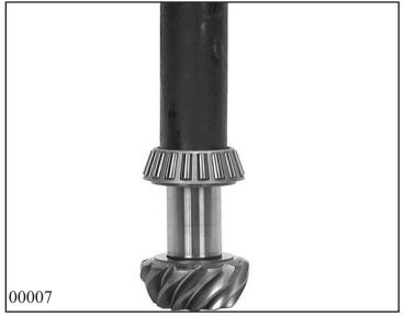
Put Setting 35.050 shim on pinion shaft. Press on inner bearing 35.020 with insertion mandrel 5x46 002 217 onto pinion shaft with mandrel press. Put on bearing shim and outer bearing race. Press on other inner bearing race with insertion mandrel 5x46 002 217 on mandrel press.
