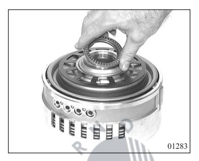
Insert complete disc set D into housing, starting with end disc 73.260 and then alternating lining disc 73.250 and outer disc 73.240. Finish with spring disc 73.230.
