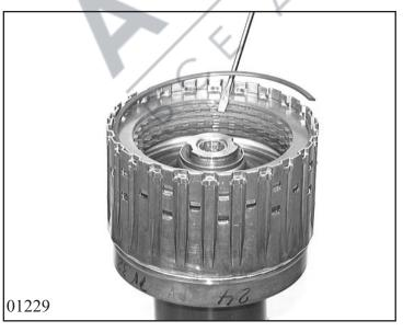
Release the snap ring of Clutch E and remove the complete disc set of Clutch E.
