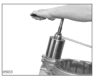
Withdraw pinion shaft from converter bell with tool 5x46 909 305. Press out shaft sealing ring of the flanged shaft from the converter bell.
