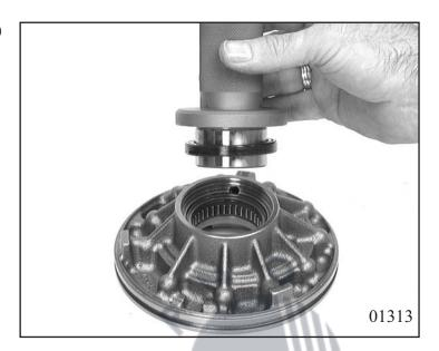
Pull on new O-ring type sealing ring 10.020.
