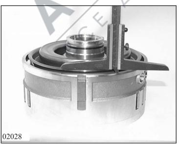
Measure down from the piston to the CD cylinder support surface and read the measured value.  $\Rightarrow$   $M_{DB}$
