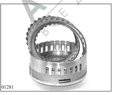
Insert complete disc set C in cylinder CD, starting with the spring disc 75.100. Then insert alternating external disc 75.140 and lining disc 75.120. Secure upper outer disc 75.160 with snap ring 73.180.
