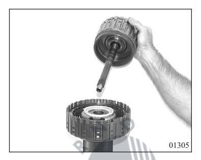
Align the discs of clutches A and E and insert intermediate shaft 71.280 while turning. Clip on axial needle bearing 71.290 onto the hub of the inner disc carrier E. Insert sun shaft 71.240 while turning.
