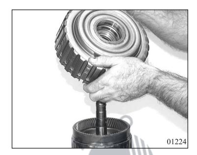
**Note!** Drive shaft is meshed with Clutch E.
