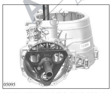
Insert the measuring part in the gearbox housing on the bearing support surface. Read the dimension  $M_R$  (plug gauge on measuring radius). Rotate the gearbox back by  $90^{\circ}$ .
