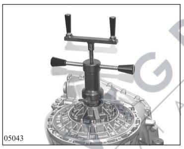
Press out oil system with jack 5x46 000 563 and remove.
