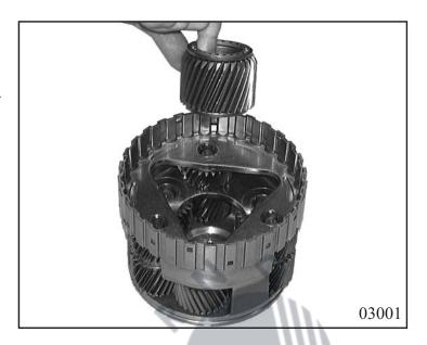
Rotate gearbox with converter bell side upwards. Clip bearing 42.210 in planetary gear set 42.010. Insert disc 42.200 and planetary gear set in gearbox housing.
