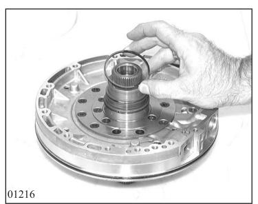
Put complete oil system on suitable support. Strip 2 rectangular rings from idler wheel shaft.
