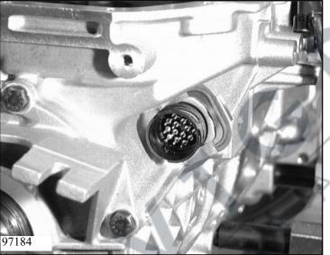
Press in the socket outlet and secure with retaining clip.
