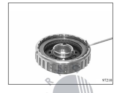
Using assembly bracket 5x46 030 167, press down cup spring C with the mandrel press, take out the split stop ring and remove the cup spring.
