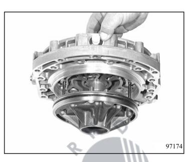
Attach shim 02.260 to the stator shaft using petroleum jelly.
