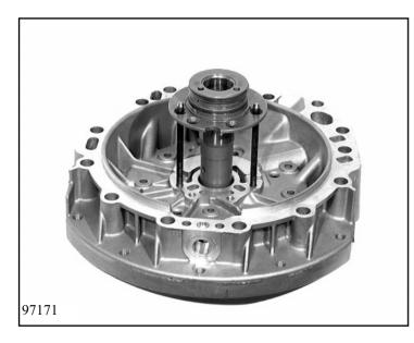
Warm the intermediate plate 10.020/110 up to 70° C using a hot-air blower. Screw two locating pins 5x46 001 007 into the intermediate plate. Guide in the stator shaft using the locating pins and secure it first with three countersunk screws 10.020/130. Remove the locating pins and screw in the rest of the countersunk screws.
