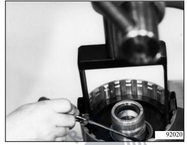
Push cylinder F out using two plastic punches.
