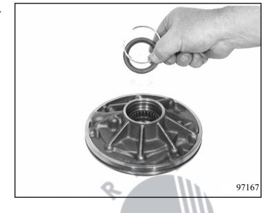
Press in sleeve 10.010/190. Assemble a new O-ring 10.014. Before putting the pump gear and pump ring gear together, lubricate them slightly with oil.
