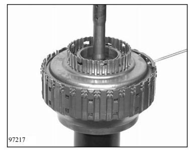
Take off clutch B from clutch A/ input shaft.
