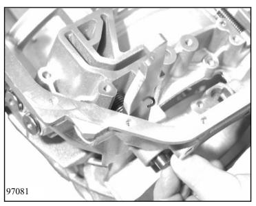
Insert pawl 01.040 and leg spring 01.050 into the transmission housing and fix it in place by pressing in bolt 01.020. Then plug up the bore using a screw plug with seal 01.090.
