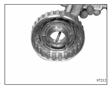
**Important!** Remove the two O-rings from the piston.
