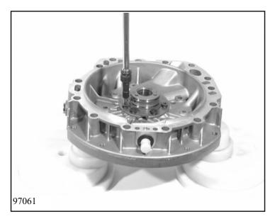
Unscrew 5 countersunk screws, warm up the housing around the stator shaft to approx.  $70^{\circ}$  C and drive the stator shaft out of the intermediate plate using the plastic-faced hammer.
