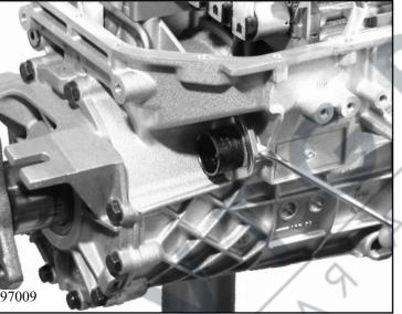
Disconnect the transport protection cap from the wiring harness socket, unlock the retaining clip using a suitable screwdriver, and press the socket into the housing by hand.
