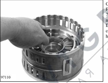
Complete cylinder DE 73.010/110. First put on two O-rings (74.010/140, 74.010/150) to the bushing 74.010/130 and press it into cylinder DE. Drive two shaft keys 73.010/140 onto the center of cylinder DE using the plastic hammer.
