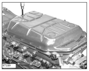
Screw plug 01.220 into the transmission housing and 03.010/130 into the oil pan.
