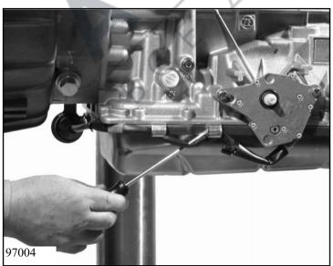
Turn the transmission 180°. Disconnect the wiring harness plug and pull it out. Remove the plug holder by unscrewing the machine screw.
