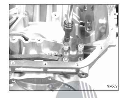
Remove the screw plug and sealing ring.
