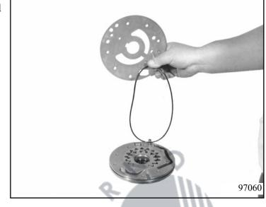
Take out the snap ring and lift out the shaft seal with a suitable screwdriver. Take out the plate.
