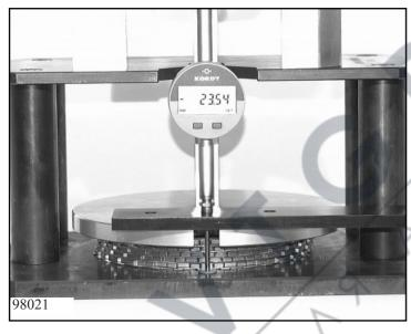
Determine thickness  $M_D$  of the brake D clutch pack according to Chapter 1.4.0: Measuring the clutch pack.
