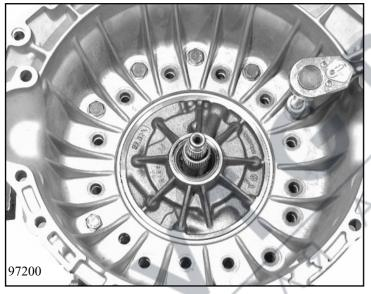
If only the converter bell housing is to be removed (damage!) unscrew the six remaining hexagonal screws and separate the converter bell housing from the intermediate plate. The intermediate plate remains on the transmission housing.
