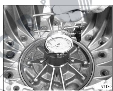
Determine axial play by pressing and pulling on the handle (repeat measurement several times)
