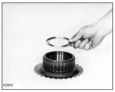
Complete first gear freewheel 77.120 by first pressing one of the freewheel's two covering washers completely into freewheel ring F.
