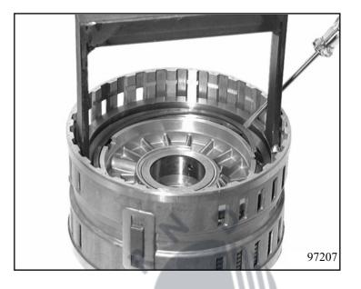
Turn over cylinder D/E, take out the brake E snap ring, and remove the complete clutch pack.
