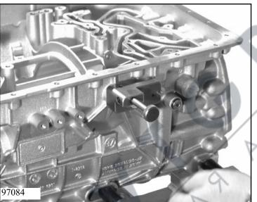
Place position gauge 5p01 002 839 on the selector shaft, turn the position gauge so that the locating pin in the transmission housing enters the cutout in the position gauge and eliminate any play by turning the knurled screw.
