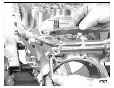
To clean the transmission housing, you have to unscrew and remove all screw plugs. These include:
