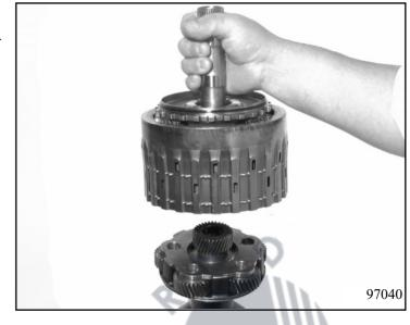
Disassemble planetary drive III by taking the sun wheel shaft out of planet carrier III.
