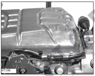
Attach cable terminals 01.490 to the oil pan.
