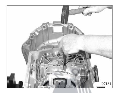
Using a suitable tool, drive in two sealing bushes 01.350 between the transmission housing and cylinder DE. Insert one 01.360 pressure spring for each sealing bushing and secure with retaining ring 01.370.
