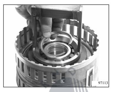
Turn over cylinder DE by  $180^{\circ}$ . Put two O-rings (73.010/152 and 73.010/154) on piston D 73.010/150 and press it into the cylinder.
