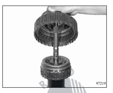
**Note!** The input shaft is meshed with clutch B.
