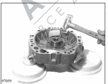
Loosen 10 machine screws (countersunk); two opposing machine screws should not be unscrewed all the way. Drive out the pump by striking these two screws carefully with a plastic-faced hammer.
