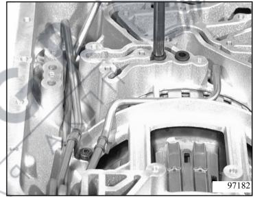
Screw testing plate 5p01 003 040 onto the control unit connection on the housing and check the function of all clutches/brakes by applying compressed air to the marked bores. Then remove the device again.
