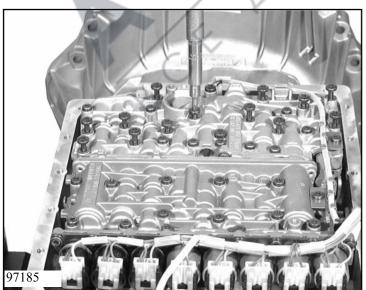
Put the detent disc in the neutral position. Align the control unit, move it into position by hand, and fasten it with 17 machine screws 27.400, and 5 machine screws 27.410.
