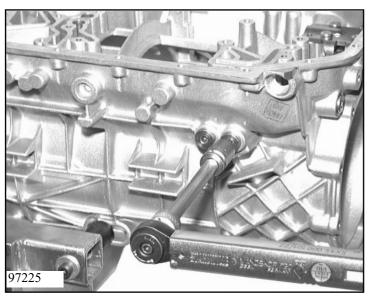
Screw new screw plugs 1x 01.650 and 2x 01.210 into the transmission housing. Insert transport plugs 01.230 and 01.240 hand-tight.
