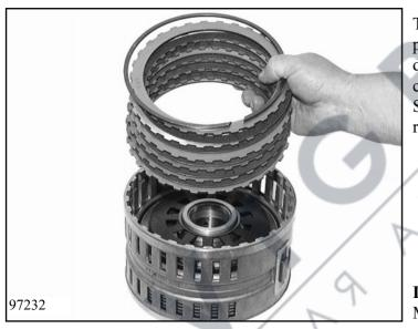
Turnover cylinder DE and insert complete clutch pack E beginning with outer disc 74.050 followed alternately by clutch lined disc 74.060 and outer disc. Secure top outer disc 74.070 with snap ring 74.090.
