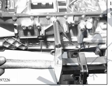
Install shaft seal 01.010/120 into the transmission housing using the drift 5x46 001 261.
