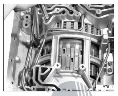
Release the two retaining rings for locking the pressure springs and remove them both.
