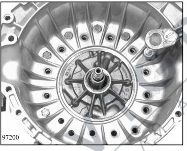
Put converter bell housing 22.010 onto the intermediate plate so that 20 hexagonal screws can be screwed in as follows: - 6 screws: 22.090 (see picture)
