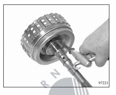
Take off the O-ring and the two rectangular-section rings from the drive shaft.
