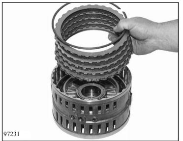
Insert the complete clutch pack D, beginning with spring clutch disc 73.010/180. This is followed by outer clutch disc 73.010/190 and lined clutch disc 73.010/200. Secure top outer clutch disc 73.010/210 with snap ring 73.010/220.
