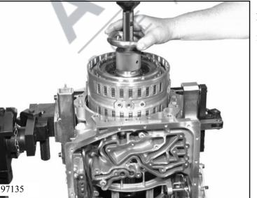
Align the bores for the oil pipes. Using a crane, carefully insert tower I into the transmission housing.
