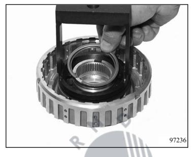
Put in complete clutch pack C beginning with spring clutch disc 75.010/170. This is followed by outer clutch disc 75.010/180 and lined clutch disc 75.010/190. Secure the top outer clutch disc 75.010/200 with snap ring 75.010/210.
