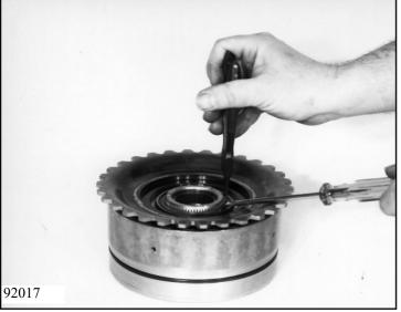
The freewheel can be separated from cylinder F as a complete unit. To do this, take out the snap ring using suitable pliers and a screwdriver, and take out the complete freewheel.
