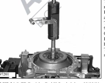
Take off the shim and the axial needle roller bearing.
