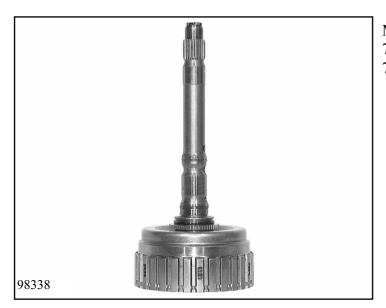
Mount 2 new rectangular-section rings 71.020 and 71.030 and new O-ring 71.150 on the input shaft.
