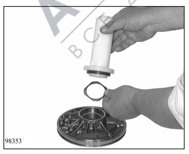
Insert disc 10.010/150 into the pump casing and mount shaft seal 10.010/160 using assembly sleeve 10.010/160.
