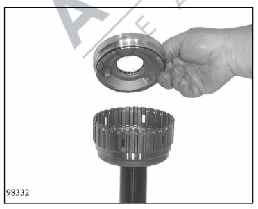
Pull new O-rings 71.060 and 71.070 onto piston E 71.050. Push piston E into cylinder E on input shaft 71.010.
