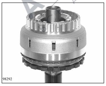
Place clutch F on the planetary drive, turning it backwards and forwards as you do so until the teeth on the lined discs and the ring gear mesh fully.
