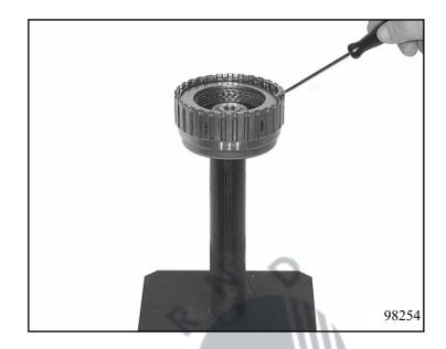
Press down the cup spring with assembly device 5x46 030 167 under a mandrel press and remove the snap ring with a suitable pair of pliers.
