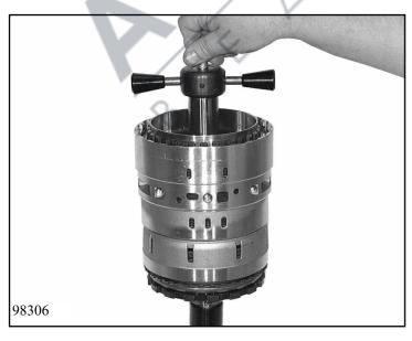
Place brake DG with 1st gear freewheel on clutch F and move backwards and forwards until the teeth on the lined discs mesh fully with the interior disc carrier. Insert lifting device 5x46 000 545 into the planet carrier of the complete planetary drive (tower). Press down the lever in the centre.
