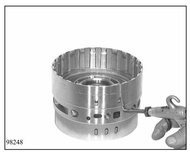
Force out piston D using compressed air in feed hole.
