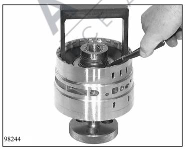
Press the cup spring down with assembly bracket 5x46 000 576 under a mandrel press.
