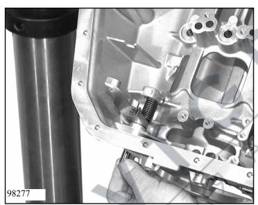
Insert pawl 01.030 and leg spring 01.040 into the transmission housing and fix them by pressing in pin 01.020. Then close the hole with screw plug 01.090.
