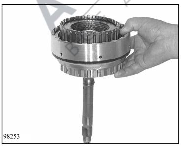
Push clutch E out of clutch A by slight pressure on the input shaft.
