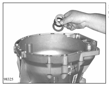
Insert thrust washer 32.060/110, axial needle roller cage 32.060/120 and angle washer 32.060/130.
