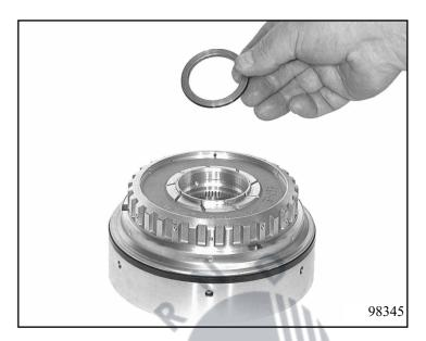
Engage clutch A in splines via the input shaft and push in as far as the stop. Next push on ring with O-ring as far as the stop.
