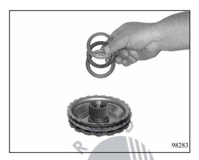
Mount planet carrier 42.010. Place the unit on supporting fixture 5x46 002 006 and secure with snap ring 42.100.
