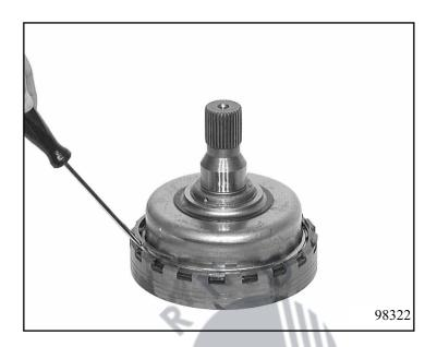
Insert angle washer 32.020/110, axial needle roller bearing 32.020/120 and thrust washer 32.020/130.
