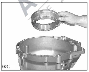
Turn the transmission by  $180^{\circ}$  and pull out lifting device  $5x46\,000\,545$  using the central handle.
