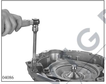
Turn transmission by 90°. Remove converter handles. Screw on converter retaining bracket 97.010 with 2 screws (97.020 and 97.030).
