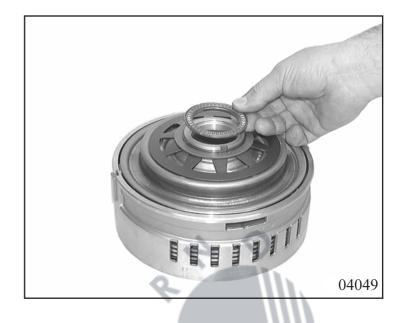
Insert complete clutch pack D into housing, starting with final disk 73.260, then insert lined disk 73.250 and external disk 73.240 alternately. Complete with spring disk 73.230.
