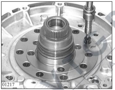
Loosen 11 machine screws (countersunk head - outer ring of stator shaft); do not take out two machine screws on opposite sides fully. Drive out the pump by striking these screws carefully with a plastic-faced hammer.
