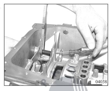
Remove the shaft sealing ring from the transmission casing with a suitable lever.
