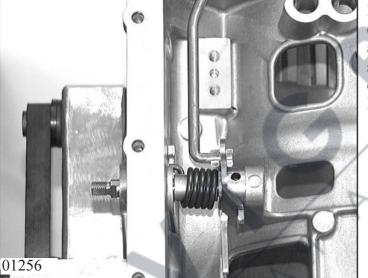
Insert parking or detent disk with connecting rod into transmission casing and push in selector shaft 06.030 through sleeve 06.070, spring 06.090 and detent disk.
