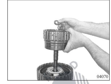
Align disks of clutches A and E and insert intermediate shaft 71.280, turning it while doing so.
