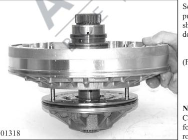
Screw locating pins 5x46 001 007 into pump. Mount complete pump over stator shaft, remove locating pins and tighten down with 11 machine screws 10.050.
