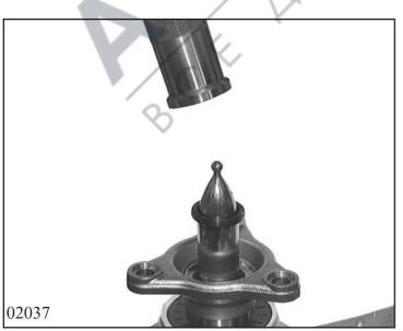
Press shaft sealing ring 14.150 into output flange 14.140 using mandrel 5x46 002 849.
