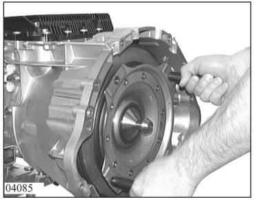
Move converter back and forward until the pump drive pins engage.
