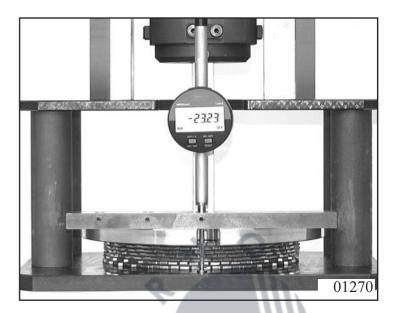
Value **P**<sub>D</sub> should be between 27.73 ■ 29.82 mm. Testing specification 1070 700 055
