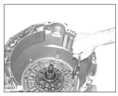
Turn transmission by 90°. Completely remove oil supply unit. To do this, loosen 14 Torx screws and remove with Usit rings.
