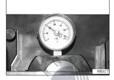
Then place measuring bar 5p01 060 330 on the measuring plate, put the dial gauge's measuring base in the measuring plate's groove on the top disc of the set, and set the dial gauge to 0.
