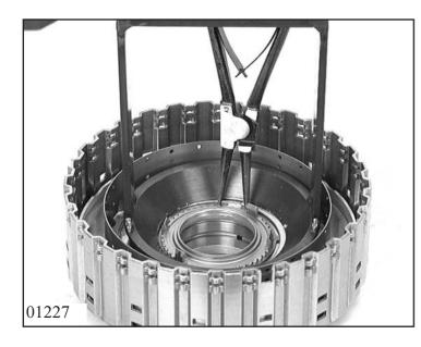
Take the O-ring seal off the baffle plate.
