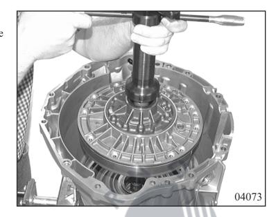
Tighten down the oil supply with 14 Torx screws and new Usit rings as follows: - 1x 10.084 (see picture) 20 mm long - 13x 10.080 (remaining screws) 50 mm long
