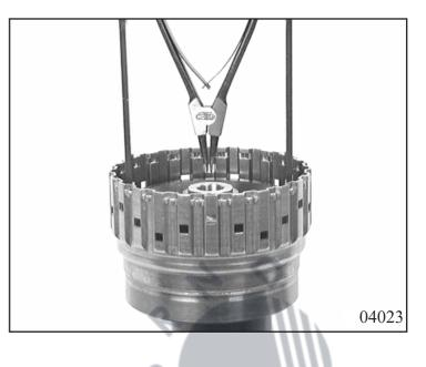
Cover one of the two oil guide bores and press out piston E with compressed air. Pull off the two O-ring seals.
