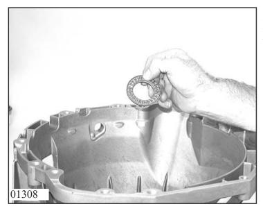
Place axial needle roller cage 72.210 on the hub of cylinder B. Note correct installed position of bearing, see picture alongside.
