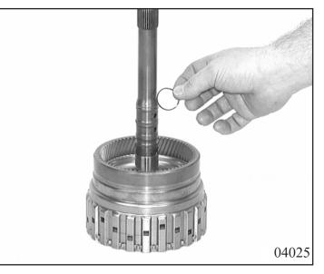
**Note!** Unclip needle roller bearing if defective.
