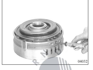
Press out piston C with the air sensor. Pull 2 O-ring off piston C.
