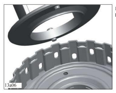
Position tool AA00 349 472 with both pins in baffle plate.
