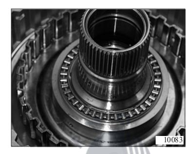
Insert disk package beginning with corrugated spring 70.120, then alternately exterior disk 70.130 and lined disks 70.140.
