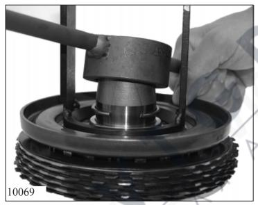
Press down the baffle plate with the pressure pad 5x46 909 248 under the mandrel press and secure it with a new round wire ring 71.140.
