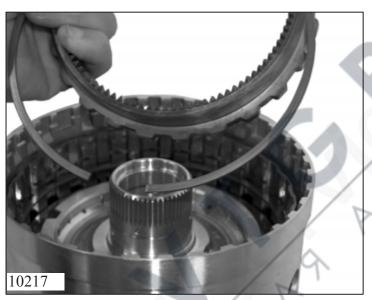
Insert internal ring gear 40.050 into the sun shaft in the position shown and secure with snap ring 40.030.
