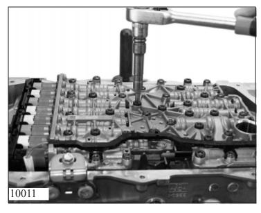
Remove 14 long screws (thick screw heads) from the mechatronic CU unit.
