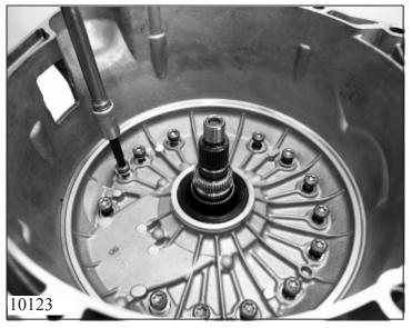
Secure the oil supply with 13 new screws 10.230.
