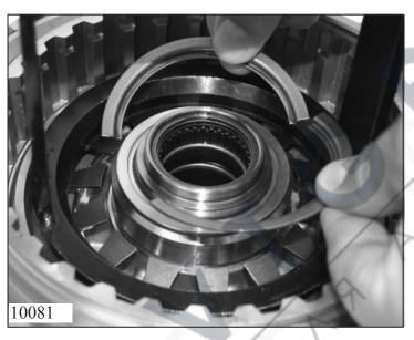
Insert disc spring 70.070 into the oil supply (cylinder A), press it down under the mandrel press using pressure pad 5x46 001 502 and secure it with a split ring 70.080.
