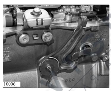
Unscrew screw for emergency release lever and remove lever.
