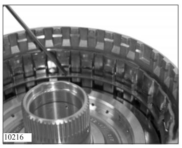
Insert new snap ring 40.070 into sun shaft.
