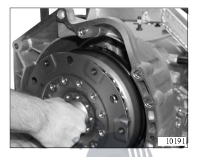
Secure the converter holder bracket 97.010 using screw 97.030 and a screw with a hexagonal nut 97.020 to the converter and transmission housing.
