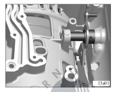
Align detent spring with centering device AA00 600 175 and tighten detent spring in this position.
