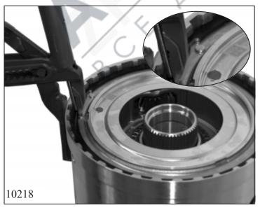
Insert planet carrier 3, 40.100, into the internal ring gear.
