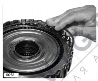
Insert the multidisc package, starting with the wave carrier 73.120, the outer clutch disc 73.140 and the lined clutch disc 73.160 alternately and the end disc 73.170.
