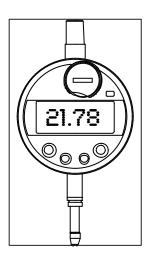
Place metering bar with dial gauge on flat surface and set dial at "zero". Fit metering bar with dial gauge on piston B and determine the depth to flat surface of intermediate plate.
