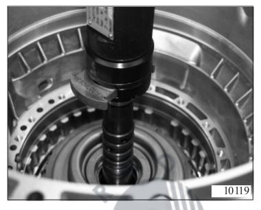
Insert brake B beginning with end disk 72.040, then alternately lined disk 72.030 and outer clutch disk 72.020, and finally spring clutch disk 72.010.
