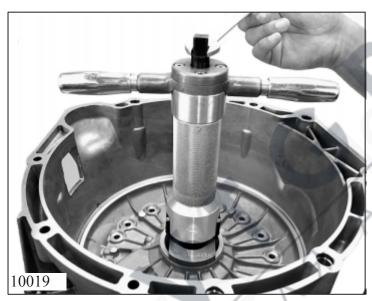
Position the lifting gear/extractor AA00 549 802 and lock with slider.
