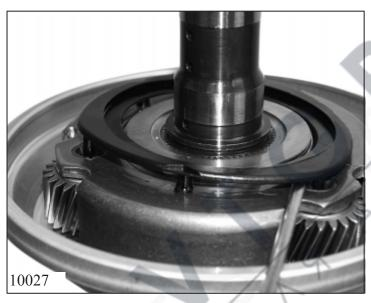
Leverage out oil tray from planet carrier 2 with screwdriver.
