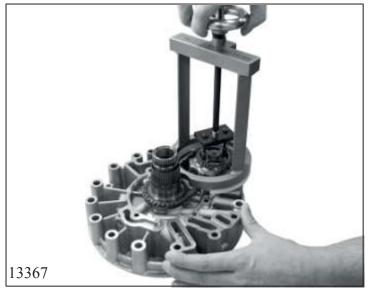
Carefully lever out and remove the pump with chain drive with tool AA00 566 429.
