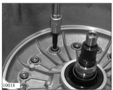
Turn transmission converter side upwards.
