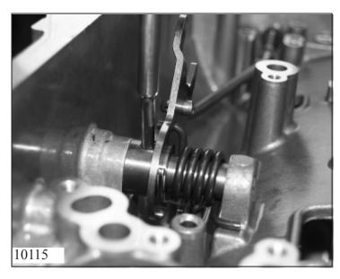
Fit new slotted spring pin 06.060 with fitting bolt AA00 524 960 in the position shown.
