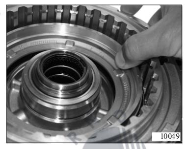
Unscrew 5 screws in cylinder A and one outside the cylinder.
