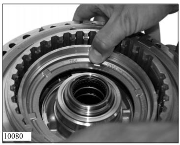
Fit 2 new lipped seal rings 70.030 and 70.050 to piston A 70.010.
