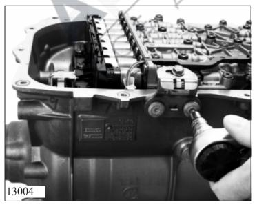
Unscrew 2 screws from the holder (emergency release puller) and remove the holder.
