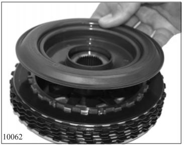
Press pist on C 75.160 on to cylinder C.
