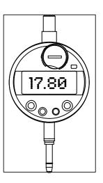
Fit metering bar with dial gauge on piston B, fit measuring sensor on piston A, set dial gauge at "zero" and determine the measurement to the upper edge of the snap ring notch.
