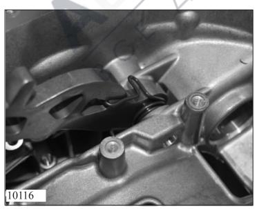
Insert the pawl 24.040 with leg spring 24.060 in the transmission housing and secure it by pressing the bolt 24.010.
