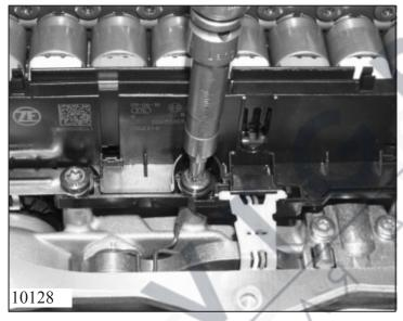
Screw in 3 screws 28.570 for the mechatronic CU unit.
