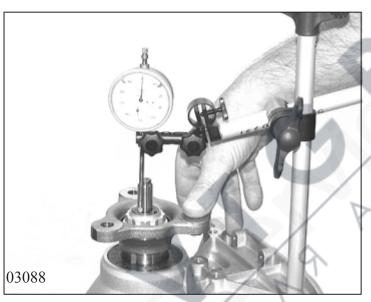
Screw measuring support 5p01 000 347 into appropriate bore in transmission casing and place dial gauge on output shaft. Press against flange and set dial gauge to
