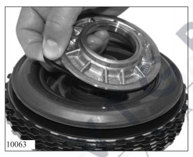
Press support plate 75.180 with a new lipped seal ring 75.200 into piston C.
