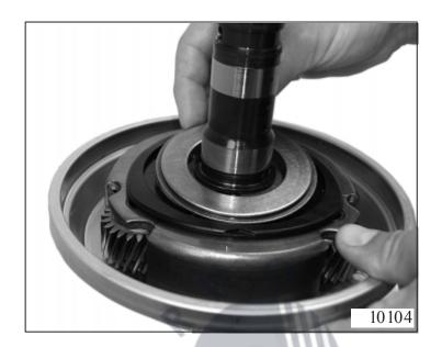
Insert input shaft into tower.
