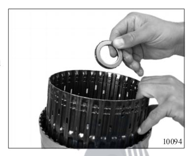
Insert clutch C into sun shaft.
