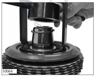
Press down the support disk with the pressure pad 5x46 909 248 under the mandrel press and secure it with a new snap ring 75.220.
