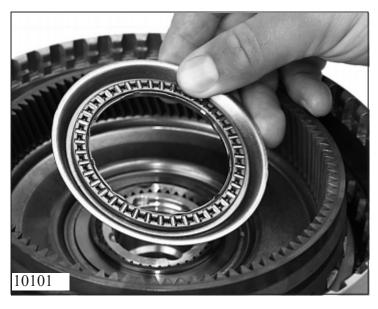
Fit needle bearing 40.170 with beveled angle washer onto sun gear.
