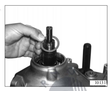
Place the output flange 14.120 on the output shaft.
