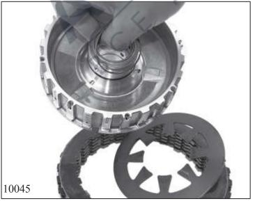
Remove the disc spring and multidisc package.
