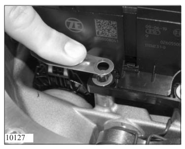
Fit a new guide sleeve 28.670 using tool AA00 548 098 and secure it with the lug.
