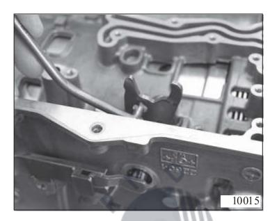
Separate connecting rod AA00 577 956 (AA00 627 091) from selector shaft.
