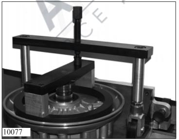
Mount centering plate and orientate according to the 13 circumferential connecting borings.
