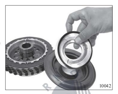
Remove the disc spring and multidisc package.
