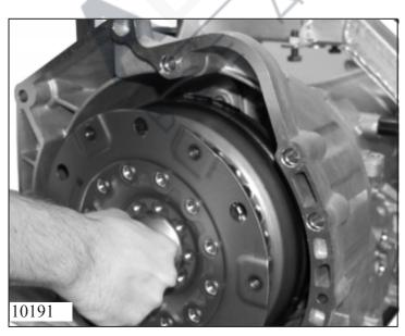
Pull out the torque converter by hand or using lifting gear 5x46 001 539 (insert meshing) and place it on one side.
