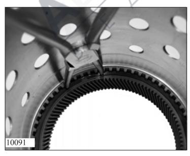
Fit the internal ring gear (gear set 4) 42.200, with the phase downwards in pot 1, 42.220.
