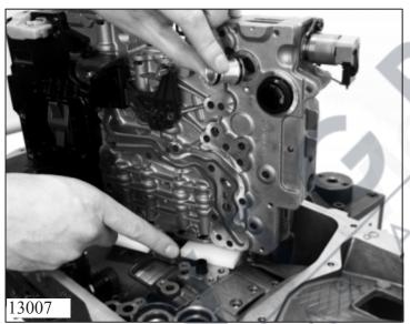
Pull the pressure pipe out of the mechatronic CU unit.
