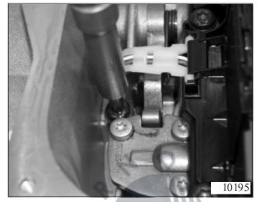
Note: Gearbox with oil volume accu = 3 screws.
