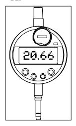
Fit metering bar with dial gauge on cylinder D, fit measuring sensor on piston D, set dial gauge on "zero" and determine measurement to upper edge of snap ring notch.
