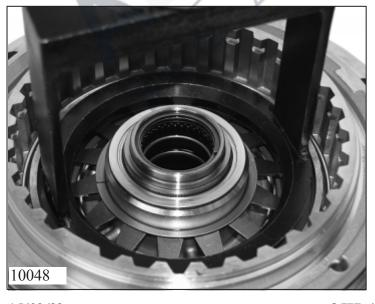
Remove the wave spring and outer clutch disc.
