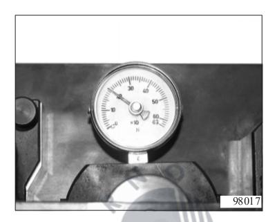
Next, place measuring bar 5p01 000 330 on the measuring plate, place the measuring foot of the dial gauge in the groove of the measuring plate on the upper disk of the disk cluster, and set the dial gauge to "0".
