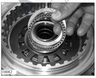
Fit a angle disc 70.100 and needle bearing 70.090 in the oil supply (cylinder A).
