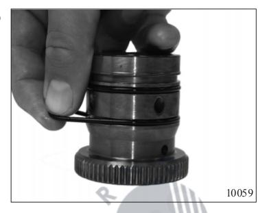
Fit the hub into cylinder C 75.050.
