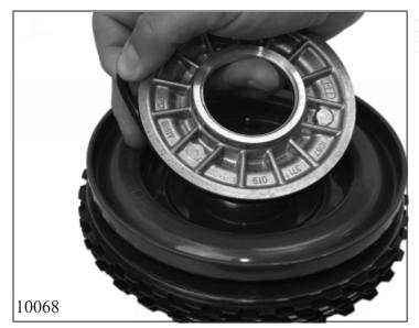
Press support plate 71.110 with a new lipped seal ring 71.120 into piston E.
