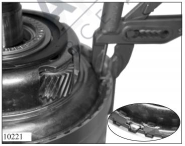
Pull pot 1 upward and secure with new snap ring 31.020.
