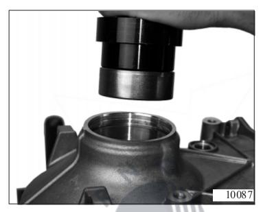
Position a new sealing sleeve 14.030 onto tool 5x54 909 281 and mount into the transmission housing.
