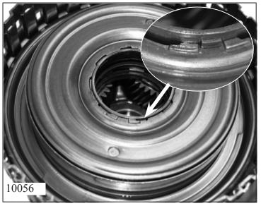
Fit new O-ring 73.100 onto baffle plate 73.080.
