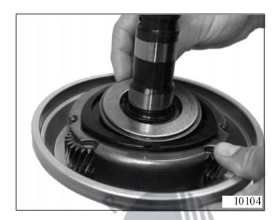
Insert input shaft into tower.
