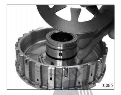
Insert disk package, beginning with end disk 71.060, and then alternately lined clutch disk 71050 and internal disk 71.040.
