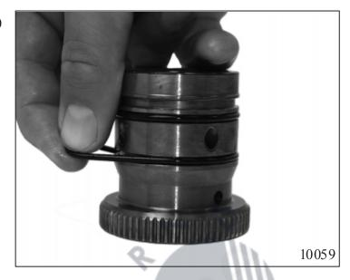
Fit the hub into cylinder C 75.050.
