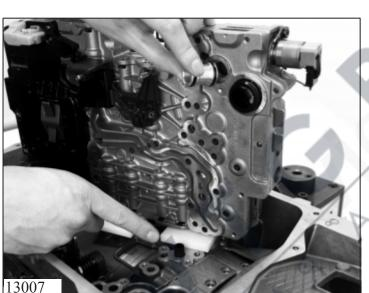
Note: Clamping effect due to pressure pipe.
