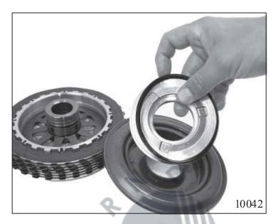
Remove the disc spring and multidisc package.
