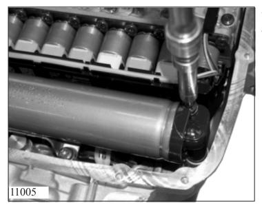
Unscrew 3 torx screws from oil volume accu.
