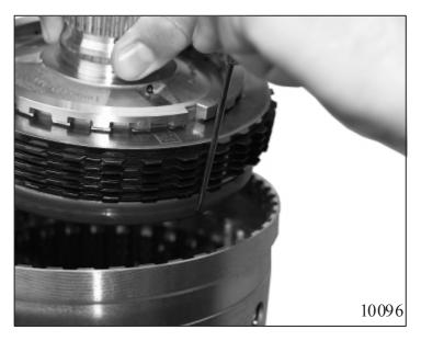
Note: Align lined disks of clutch E before insertion.
