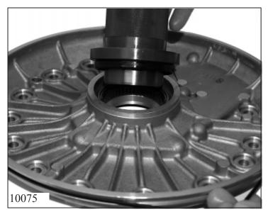
Fit a new O-ring 10.200 on the centring plate, press the shaft sealing ring 10.100/140 into the centring plate using tool AA00 613 946.
