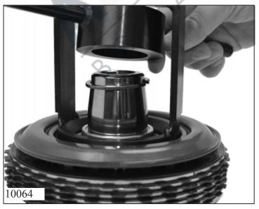
Press down the support disk with the pressure pad 5x46 000 167 under the mandrel press and secure it with a new snap ring 75.220.
