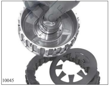
Remove the disc spring and multidisc package.
