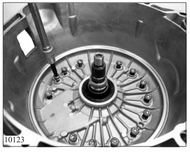
Secure the oil supply with 14 new screws 10.230.
