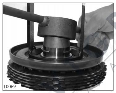
Press down the baffle plate with the pressure pad 5x46 000 167 under the mandrel press and secure it with a new round wire ring 71.140.
