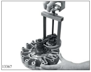
Carefully lever out and remove the pump with chain drive with tool AA00 566 429.
