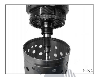
Insert finished pot 2 into pot 1 while rotating.
