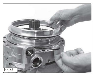
Mount new O-ring 72.140 onto intermediate plate.
