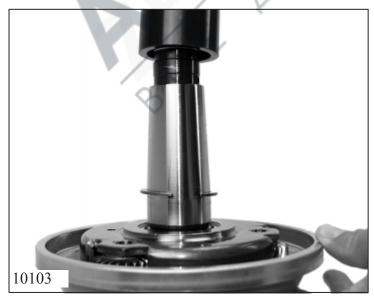
Secure planet carrier with new snap ring 32.050.
