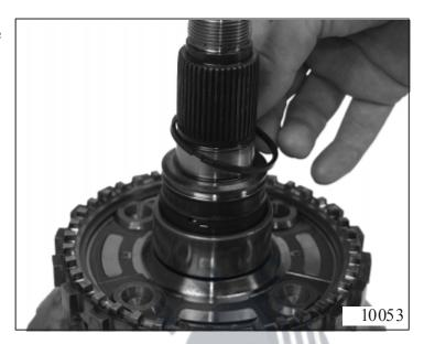
Insert the output shaft in the mounting device.
