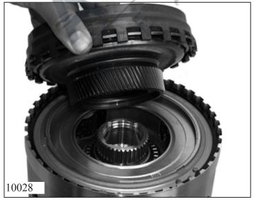
Remove internal ring gear 2 with sun gear 3 from pot 2.
