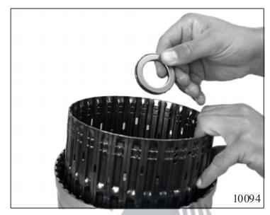
Insert clutch C into sun shaft.
