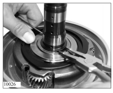
Leverage out thrust washer from planet carrier 2.
