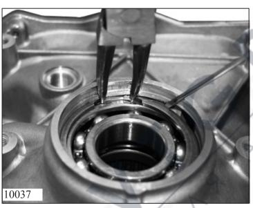
Remove the snap ring from the ball bearing.
