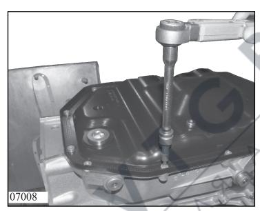
Fix gasket 03.050 on sealing surface. Put oil pan 03.010/110 and fix with screws 03.020/010.
