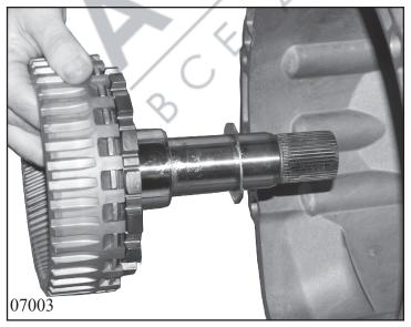
Install output shaft 42.190 into internal gear 42170 and secure with circlip 42.180.
